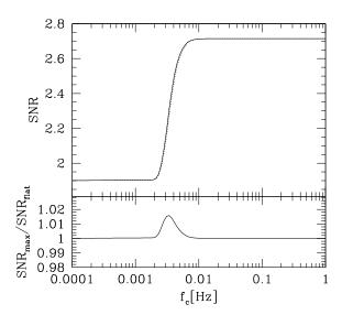
FIG. 4: The value (top) and ratio (bottom) of SNRs for  $\Omega_{\rm filter} = \Omega_{\rm gw}$  (solid line in top panel) and  $\Omega_{\rm filter} \propto f^0$  (dotted line in top panel) for LISA. We set d=0.7.
