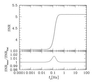
FIG. 3: The value (top) and ratio (bottom) of SNRs for  $\Omega_{\rm filter} = \Omega_{\rm gw}$  (solid line in top panel) and  $\Omega_{\rm filter} \propto f^0$  (dotted line in top panel) for FP-DECIGO. We set d = 0.7.
