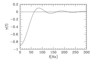
FIG. 1: The overlap reduction function  $\gamma(f)$  for the Hanford and Livingston, LIGO detector pair.
