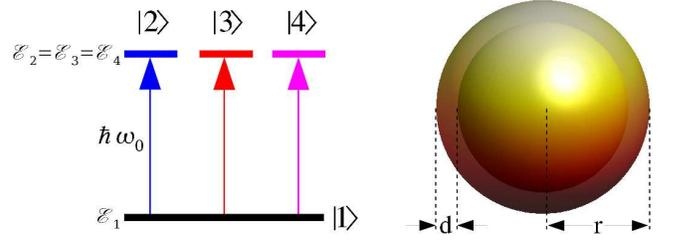
FIG. 1: (Color online). (left) Energy diagram of a four-level atomic system with a triply-degenerate excited state; (right) sketch of a single Mie nanoresonator with a  $d$ -thick layer of amplifying material.
