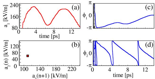
FIG. 4: (Color online). Frequency demodulation analysis: time evolution of modal amplitude  $a_1(t)$  (a) and phases  $\phi_{1,2}(t)$  (c-d); (b) 1D map obtained with a Poincaré surface of section of  $(a_1, a_2)$  at  $a_1 = 180 \text{ kV/m}$ .
