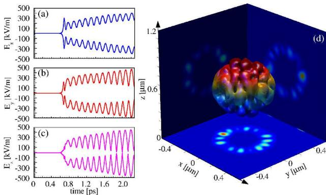
FIG. 2: (Color online). MB-FDTD results for  $N_a = 10^{26} \text{ m}^{-3}$ : (a)-(c) time evolution of the electric field components (sampled in proximity of the sphere center, to avoid symmetry effects), (d) energy density  $\mathcal{E}$  (isosurface plot) with  $xy$  (down)  $xz$  (left) and  $yz$  (right) slices in the sphere middle plane.
