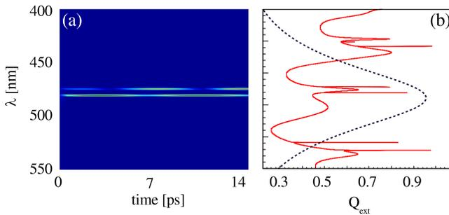
FIG. 3: (Color online). (a) Time series spectrogram computed from MB-FDTD analysis for  $N_a = 10^{26} \text{ m}^{-3}$  (the mode-competition dynamics is denoted by the beating mode-amplitudes); (b, solid line) Mie theory extinction factor  $Q_{ext}$  for a single nanosphere of diameter 600 nm and  $\epsilon_r = 8.41$ ; (b, dashed line) active medium gain bandwidth.
