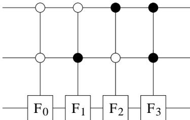
FIG. 2: A quantum circuit implementing a generic diagonal unitary transformation (14), for the case of  $n = 3$  qubits. Empty or full circles indicate that the operation on the target qubit is active only when the control qubits are set to 0 or 1, respectively.
