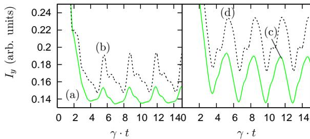
FIG. 8: (Color online) Time dependence of the fluorescence intensity averaged over  $\theta$  with fixed inter-atomic distance  $r_{12} = 0.1\lambda$ . (a) AC method with  $\phi = 0.6\pi$ , (b) AP method with  $\phi = 0.6\pi$ , (c) AC method with  $\phi = 0.9\pi$ , and (d) AP method with  $\phi = 0.9\pi$ . The other parameters are as in Fig. 2.
