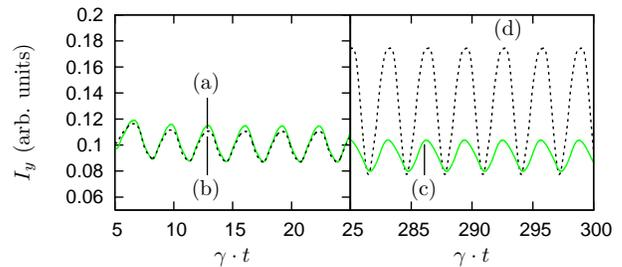
FIG. 6: (Color online) Comparison of the time dependence of the fluorescence averaged over  $r$  by both methods. The orientation angles  $\theta = 0.5\pi$  and  $\phi = 0.25\pi$  are fix and  $r_m = 0.25\lambda$ . (a) AC method,  $r_a = 0.14\lambda$ , (b) AP method,  $r_a = 0.14\lambda$ , (c) AC method,  $r_a = 0.2\lambda$ , (d) AP method,  $r_a = 0.2\lambda$ . All other parameters are as in Fig. 2.
