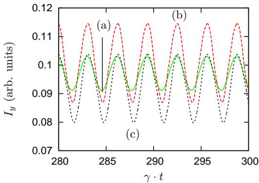
FIG. 2: (Color online) Time dependence of the fluorescence intensity averaged over  $r_{12}$  by the AC method.  $r_m = 0.25\lambda$  and (a)  $r_a = 0.02\lambda$ , (b)  $r_a = 0.14\lambda$  and (c)  $r_a = 0.2\lambda$ . The inter-atomic distance vector is oriented such that  $\phi = \pi/4$  and  $\theta = \pi/2$ . The laser parameters are  $\Omega_1 = 3\gamma$ ,  $\Omega_2 = 5\gamma$ ,  $\Delta_1 = 0$ ,  $\Delta_2 = 2\gamma$ , and the two lower states are assumed degenerate  $\delta = 0$ .
