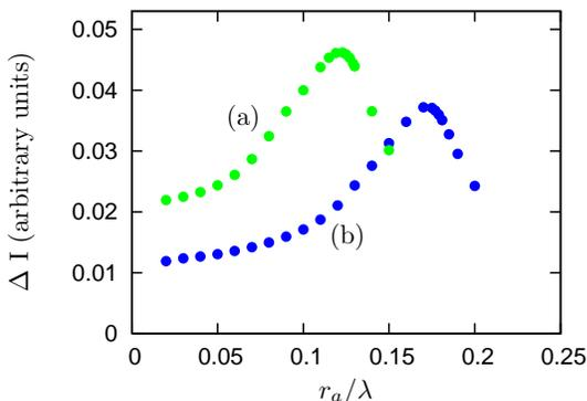
FIG. 3: (Color online) Dependence of the amplitude of the oscillating fluorescence intensity on the oscillation amplitude  $r_{12}$  of the atom for (a)  $r_m = 0.2\lambda$  and (b)  $r_m = 0.25\lambda$ . The other parameters are as in Fig. 2.
