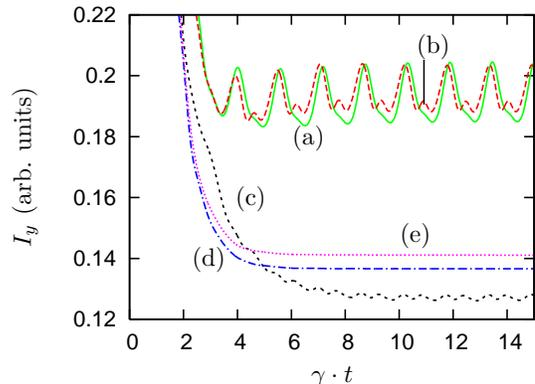
FIG. 9: (Color online) Time dependence of the fluorescence intensity averaged over  $\phi$ .  $r_{12}$  is fixed at  $0.1\lambda$ . (a)  $\theta = 0.25\pi$ , (b)  $\theta = 0.3\pi$ , (c)  $\theta = 0.5\pi$  and (d)  $\theta = \pi$ . Curves (a-d) are obtained using the AC method. (e) shows a result using the AP method for  $\theta = 0.3\pi$ . All other parameters are as in Fig. 2.
