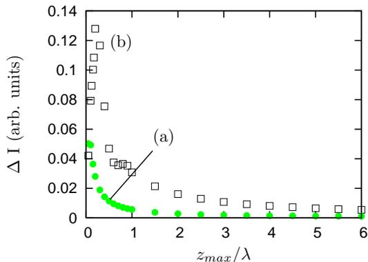
FIG. 13: (Color online) Dependence of the oscillation amplitude of the time-dependent intensity on  $z_{max}$  for impact parameter  $r_{min} = 0.05\lambda$ .  $\phi = \pi/4$ , and the other parameters are as in Fig. 2. In (a) we used the AC and in (b) the AP method.
