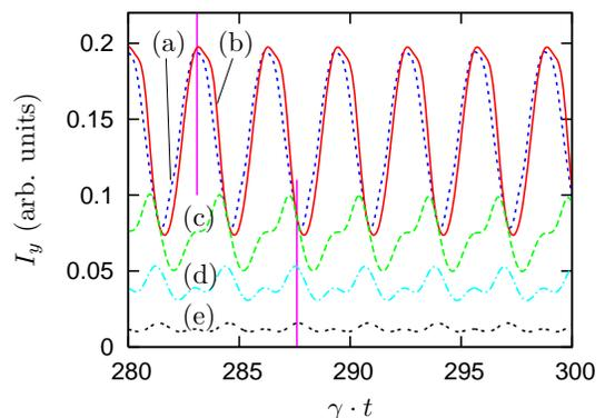
FIG. 4: (Color online) Time-dependent fluorescence signal for different fixed distances  $r_{12}$  without any averaging. (a)  $r_{12} = 0.10\lambda$ , (b)  $r_{12} = 0.08\lambda$ , (c)  $r_{12} = 0.06\lambda$ , (d)  $r_{12} = 0.05\lambda$ , (e)  $r_{12} = 0.04\lambda$ . The other parameters are as in Fig. 2. The vertical lines allow to easily judge the relative phase shifts of the different curves.
