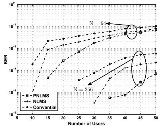
Fig. 3. The BER of the conventional, the modified LMS-PPIC and the modified PLMS-PPIC methods versus the system load in time varying Rayleigh fading channel, using two stages for  $N = 64$  and  $N = 256$ .
