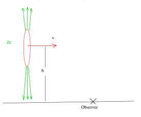
Figure 1: A fast charged particle moving on a straight line with impact parameter b causes a time-dependent electromagnetic field at the point of the observer. This field corresponds to a spectrum of equivalent photons.
