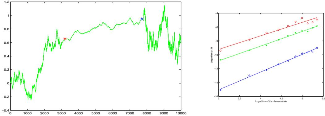
Figure 5: (left) Detection of the change point in piecewise FBM( $H_j$ ) ( $\tau_1 = 0.3$ ,  $\tau_2 = 0.78$ ,  $H_0 = 0.6$ ,  $H_1 = 0.8$  and  $H_2 = 0.5$ ). The change points estimators are  $\hat{\tau}_1 = 0.32$  and  $\hat{\tau}_2 = 0.77$ . (right) Representation of log-log regression of the variance of wavelet coefficients on the chosen scales for the three segments ( $\tilde{H}_0 = 0.5608$  (\*),  $\tilde{H}_1 = 0.7814$  ( $\triangleleft$ ) and  $\tilde{H}_2 = 0.4751$  (o))
