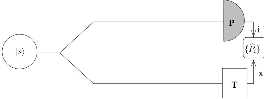
FIGURE 3. Experimental set-up to determine the POVM associated to an unknown photometer  $\mathbf{P}$ . We use it to measure a known bipartite state  $|s\rangle$ , jointly with a tomographer  $\mathbf{T}$ . The photometer gives a result  $i$  and the tomographer a result  $x$ . From these samples, we construct an estimator  $\{\hat{P}_i\}$  of the self-adjoint operators associated to the results  $\{i\}$  by the photometer  $\mathbf{P}$ .
