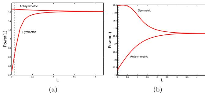
FIG. 6: (Color online) The total power of the antisymmetric and symmetric narrow (a) and broad (b) solitons as a function of thickness  $L$  of the buffer layer between the channels. Fixed parameters are  $V_0 = 3$ ,  $D = 8$ , and  $k = 3.1$ . The dashed vertical lines mark small values of  $L$  at which the stability is switched, see text.
