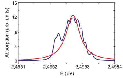
FIG. 3: (Color online) Absorption spectrum in the vicinity of the lower polariton energy calculated exactly (blue) and within the perturbation theory and broadened by Lorentzian (red) with  $\Gamma = 5$  eV. 40 Realizations of energy disorder with variation  $\sigma = 1$  m eV on the lattice with  $20^2$  sites were considered.
