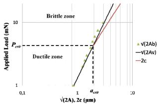
Figure 5: Comparison between plastic deformation sizes induced by nanoindentation and Vickers indentation on CaCO<sub>3</sub> for single-cycle study
