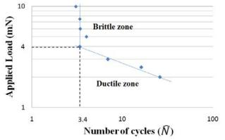
Figure 6: Wöhler diagram of the contact fatigue results
