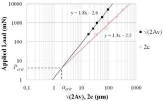
Figure 4: Vickers indentation results: plasticity length  $\sqrt{2}A_{\nu}$  (solid squares), fracture 2*c* (open circles). Extrapolations of these results give the critical size of CaCO<sub>3</sub>
