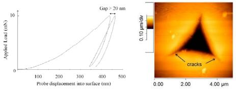
Figure 2: a) Indentation curve on CaCO<sub>3</sub>, b) Corresponding AFM image of the Berkovich indent with cracks (maximum load = 10 mN)
