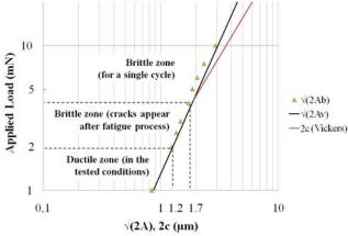
Figure 7: Evolution of the brittle-ductile transition with fatigue
