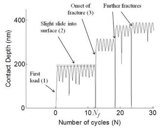
Figure 3: Contact depth as a function of the number of cycles (*N*) for a maximum load = 2.5 mN (here cracking occurs for  $N_f = 12$ ). Further fractures are often observed after the first one occurred.
