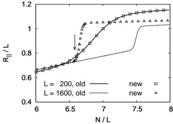
FIG . 16: A average end-to-end distance divided by  $L$ ,  $R_{jj}=L$ , plotted against  $N=L$  for  $L = 200$  and  $600$ , and  $D = 21$ . Results are obtained by PERM with (new) and without (old) force biases. The true transition point is indicated by an arrow .
