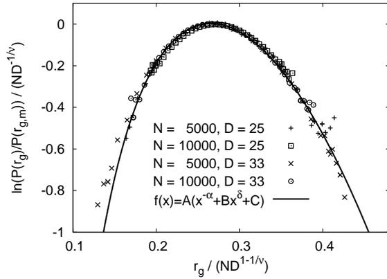
FIG. 6: Rescaled distribution  $\ln(P(r_g;N;D)/P(r_{g,m};N;D))=(ND^{-1/\nu})$  plotted against  $r_g/ND^{-1/\nu}$  for various values of  $N$  and  $D$ . The radius of gyration  $r_{g,m}$  corresponds to the maximum of the distribution  $P(r_g;N;D)$ . Near  $r_{g,m}$ ,  $f(x) = A(x^{-\alpha} + Bx^\delta + C)$  with  $A = 0.185$ ,  $B = 76.757$ , and  $C = 8.784$  gives the best fit of the data, here  $x = r_g/(ND^{-1/\nu})$ .
