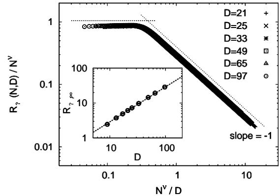
FIG. 4: Rescaled rms end-to-end distance perpendicular to the tube,  $R_{\perp}(N; D)/N$ , plotted against  $\cdot = N/D$ . The data collapse is achieved by Eq. (4) and corrections to scaling are not visible in a log-log scale. The inset shows the log-log plot of  $R_{\perp, \lim} = \lim_{N \rightarrow \infty} R_{\perp}(N; D)$  versus  $D$ . The dashed line is  $0.295D^{-1}$ .
