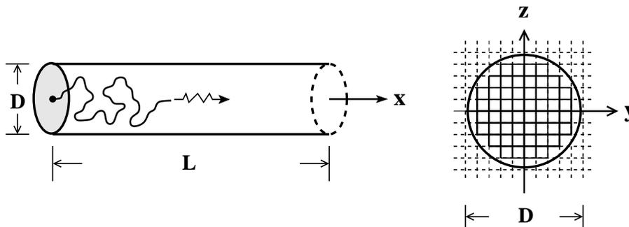
FIG. 2: Schematic drawing of a one-end grafted polymer chain growing as a self-avoiding walk inside a finite tube of length  $L$  and diameter  $D$  along the  $x$ -direction. The first monomer is located at  $(x = 0; y = 0; z = 0)$ . Other monomers are allowed to sit on lattice sites of a simple cubic lattice, except for the lattice sites representing the cylindrical walls for  $0 < x < L; y^2 + z^2 = D^2/4g$  and the bottom  $z = 0; y^2 + z^2 < D^2/4g$ .
