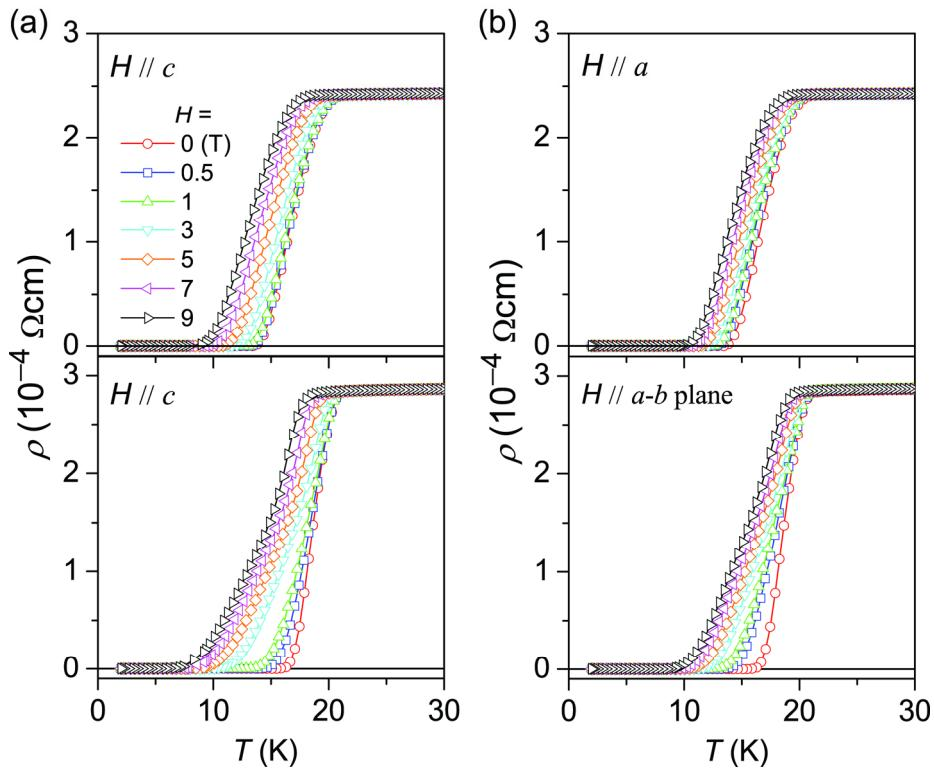
Fig. 3. Superconducting transitions under magnetic fields ( $H$ ) varying from 0 to 9 T applied parallel to the  $c$ -axis (a) and the  $a$ -axis of the LSAT substrates (b). The top and bottom panels correspond to the HQ and LQ films, respectively.
