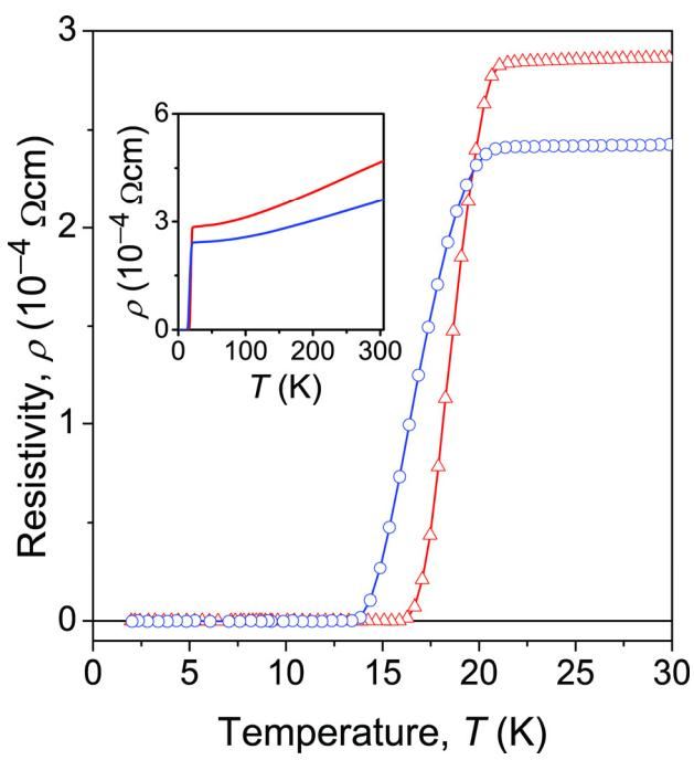
Fig. 2. Temperature dependencies of electrical resistivities of the Co-doped  $\text{SrFe}_2\text{As}_2$  thin films. Inset shows expanded views between 2 and 305 K. Blue circles and red triangles show the HQ and LQ films, respectively.
