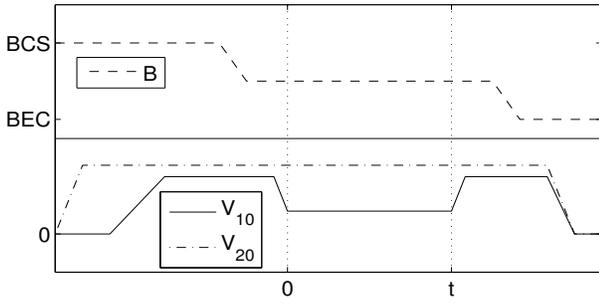
FIG. 1: The time sequences for the magnetic field ( $B$ ) and the lattice potentials ( $V_{10}$  and  $V_{20}$ ) to achieve state preparation, controlled dynamics, and detection. (Note that the optical barriers are high during sweeping of the  $B$  field.)
