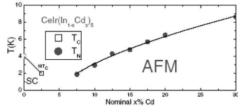
FIG. 11: Phase diagram of the heavy fermion  $\text{CeIr}(\text{In}_{1-x}\text{Cd}_x)_5$ . The figure is extracted from Ref. 9.
