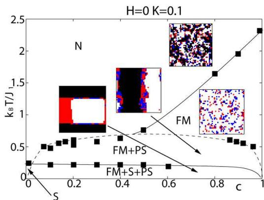
FIG. 2: (color online) Phase diagram in the absence of a magnetic field, for a relative coupling constant of  $K = 0.1$ .
