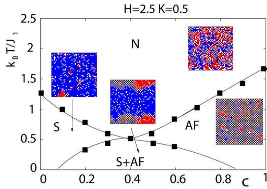
FIG. 4: (color online) Phase diagram at a magnetic field  $H = 2.5$  and relative exchange strength  $K = 0.5$ . There is a region where superconductivity and antiferromagnetism coexist, but where there is no true phase separation.
