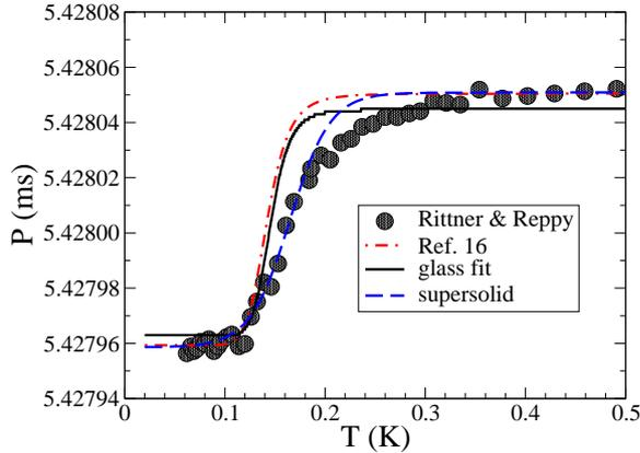
**Figure 4.** Change in resonance period  $P$  [2]. Both glass and supersolid model can explain the observed change. Fit parameters for glass are  $A = 0.0390 \text{ s}^{-1}$ ,  $f_0 = 184.23119 \text{ Hz}$ ,  $Q_\infty^{-1} = 11.33 \cdot 10^{-6}$ ,  $\tau_0 = 0.360 \mu\text{s}$ ,  $\Delta = 1.135 \text{ K}$ .
