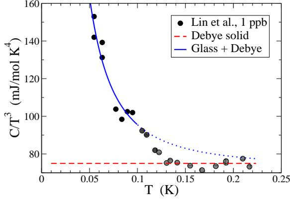
**Figure 1.**  $C/T^3$  of ultra-pure (1 ppb of  $^3\text{He}$ ) solid  $^4\text{He}$  from Lin et al. [12]. The non-Debye behavior below  $T_c \approx 0.12$  K signals the freezing out of two-level systems.
