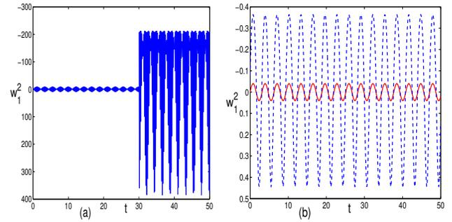
FIG. 5: (color online) The trapping frequency varies with time when the field varies periodically with time. (a)  $m = 0.01$  ( $0 < t < 30$ ),  $m = 0.3$  ( $30 < t < 50$ ), and  $w = 30$  for the case with atomic attractive interaction. (b)  $m = 0.01$  (red solid line),  $m = 0.1$  (blue dashed line), and  $w = 2$  for the case with atomic repulsive interaction. The frequency is measured in units of  $w_2^2$ .
