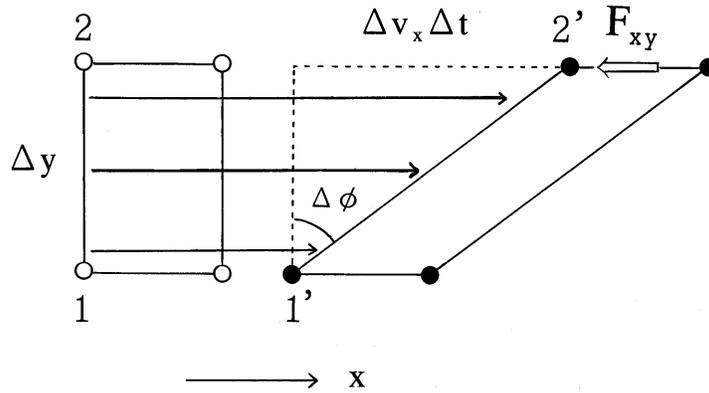
FIG. 6: In a liquid flowing along the x-direction, owing to the velocity gradient along the y-direction, a small rectangular part of a liquid is deformed to a parallelogram.
