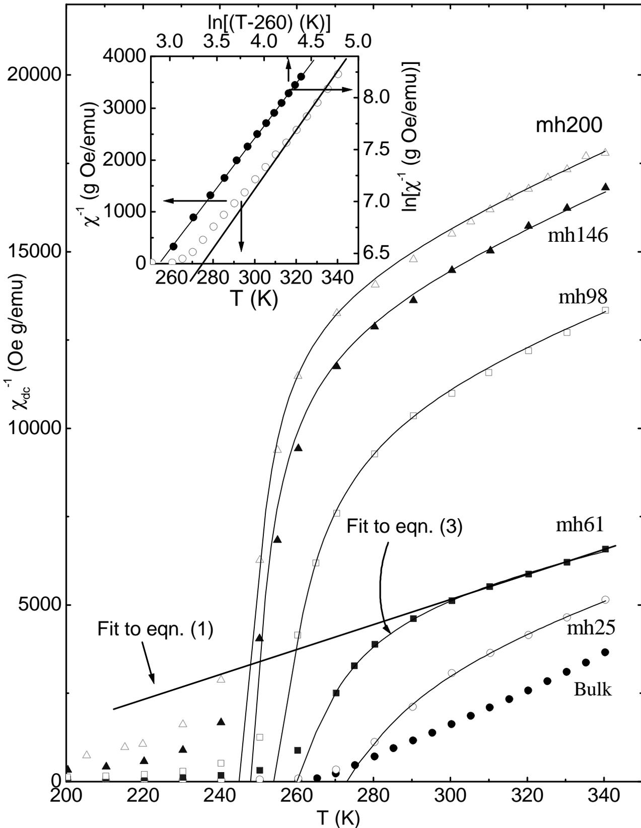
Fig. 6. (Colour online) Inset shows the  $\chi^{-1}$  vs. temperature data for bulk sample fit with eqn. (1) (straight line) (left-bottom scale) and fit with eqn. (2) (right-top scale). Main panel shows the experimental data with non-linear fit to eqn. (3).
