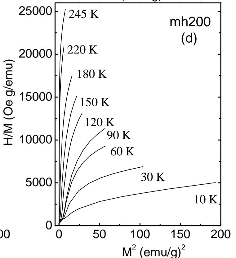
Fig. 9. (a) Normalized ( $M^2$  vs.  $H/M$ ) plot at 10 K for selected samples, along with line and polynomial fit to calculate spontaneous magnetization. (b-d)  $H/M$  vs.  $M^2$  plot for bulk, mh61 and mh200 samples. The dotted lines indicate the slope at  $H = 0$  limit.
