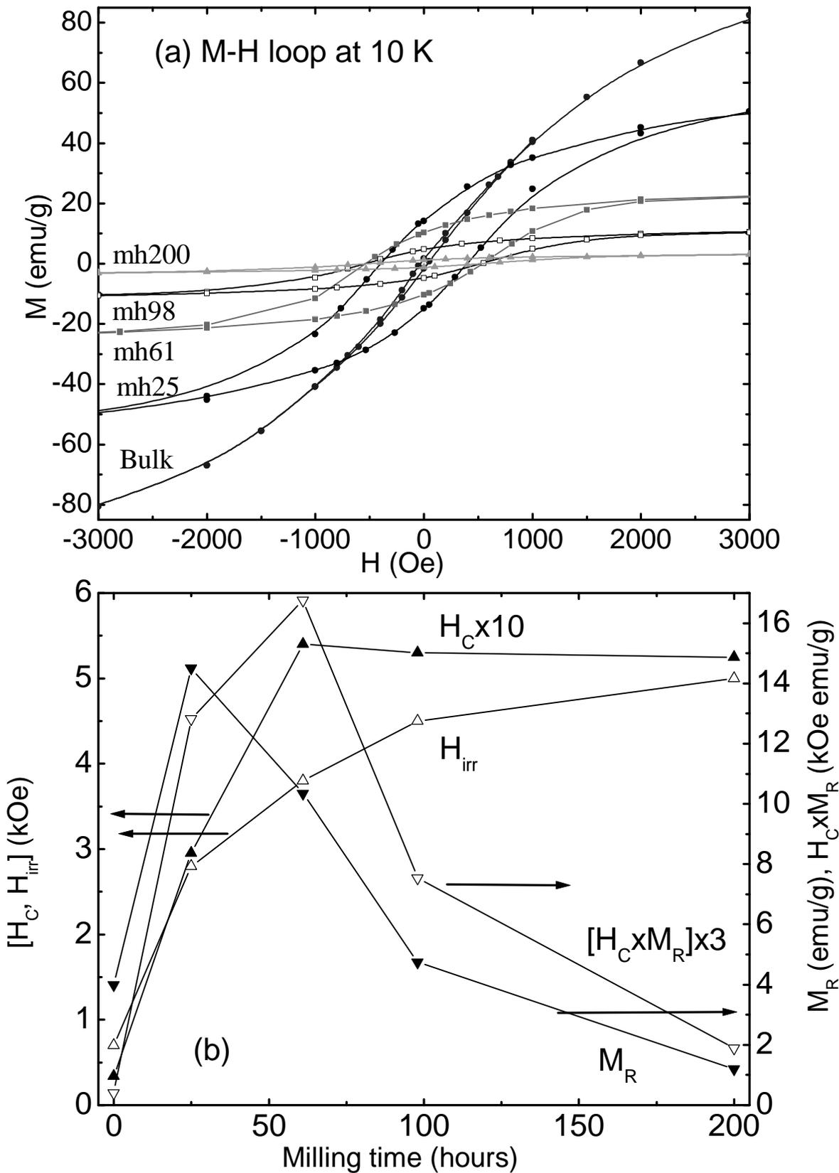
Fig. 7 (a) (Colour online) M-H loop at 10 K for different samples and corresponding magnetic parameters with milling time in (b), where  $H_C$  is coercive field,  $H_{irr}$  is irreversibility field,  $M_R$  is remanent magnetization and  $H_C \times M_R =$  energy product.
