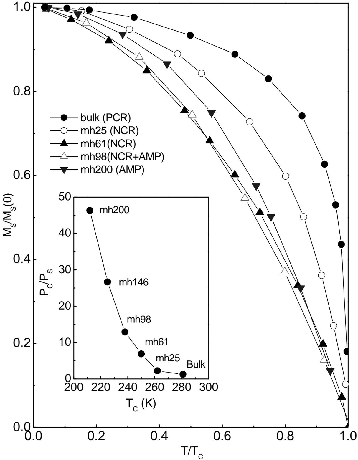
Fig. 10 (Colour online) The reduced plot ( $M_s(T)/M_s(0)$  vs.  $T/T_c$ ) for selected samples. The inset shows Rhodes-Wohlfarth plot ( $P_c/P_s$  vs.  $T_c$ ) for the samples.  $P_c$  and  $P_s$  are derived from the effective magnetic moment ( $P_{\text{eff}}(\mu_B)$ ) and  $M_s(0)(\mu_B)$  per formula unit. The notations: PCR, NCR and AMP are mentioned in Table 1.
