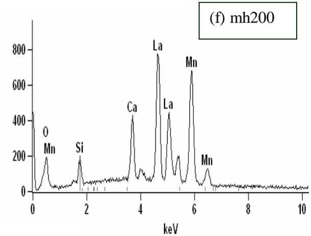
FIG. 2: SEM pictures for bulk (a), mh61 (b) and mh200 (c) samples, and corresponding EDAX spectrum for bulk (d), mh61 (e) and mh200 (f) samples.
