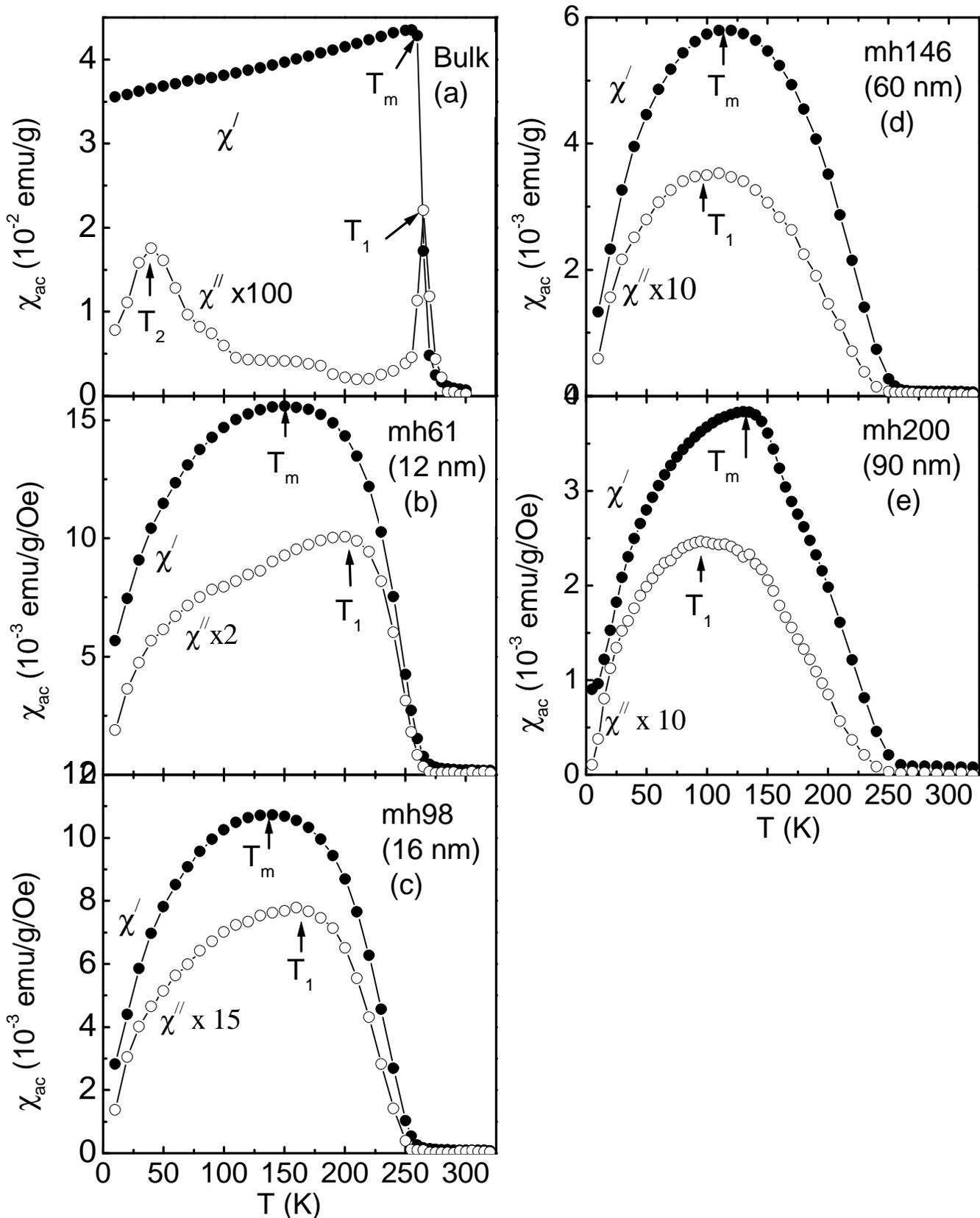
Fig. 3 ac susceptibility data at 1 Oe and 10 Hz for  $\text{La}_{0.67}\text{Ca}_{0.33}\text{MnO}_3$  samples.  $T_m$  and  $T_1$  shows the peak positions for  $\chi'$  and  $\chi''$ , respectively.  $T_2$  represents the low temperature  $\chi''$  peak position for bulk sample. Note that  $\chi''$  data are multiplied by some factor.
