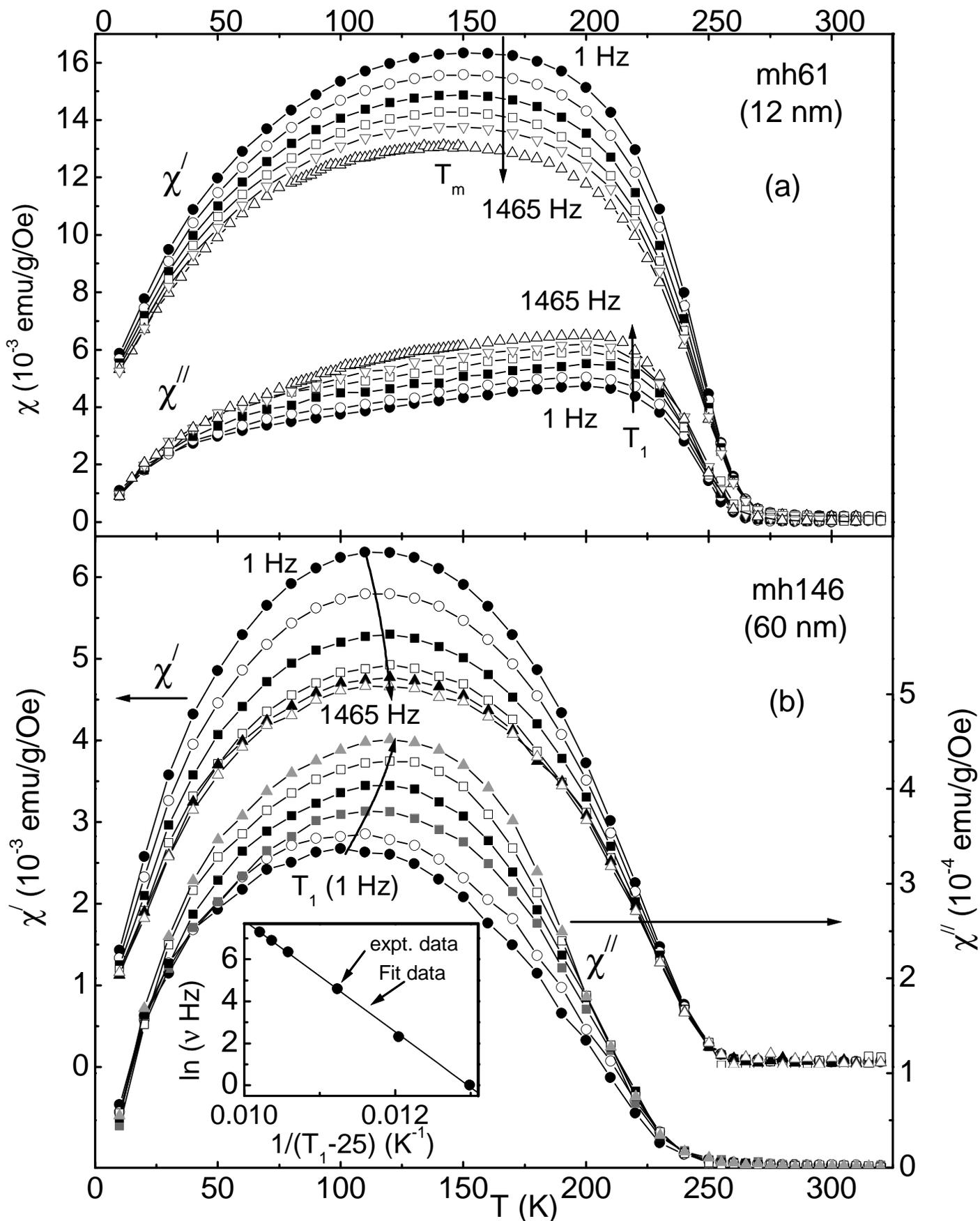
Fig. 4 (Colour online) ac susceptibility ( $\chi'$ ,  $\chi''$ ) data for mh61 (a) and mh146 (b) at  $\nu = 1$  Hz, 10 Hz, 99 Hz, 575 Hz, 997 Hz and 1465 Hz. The arrows guide the shift of ( $\chi'$ ,  $\chi''$ ) maximum as  $\nu$  increases from 1 Hz to 1465 Hz. Inset (b) shows the fit of  $T_1(\nu)$  data to Vogel-Fulcher law.
