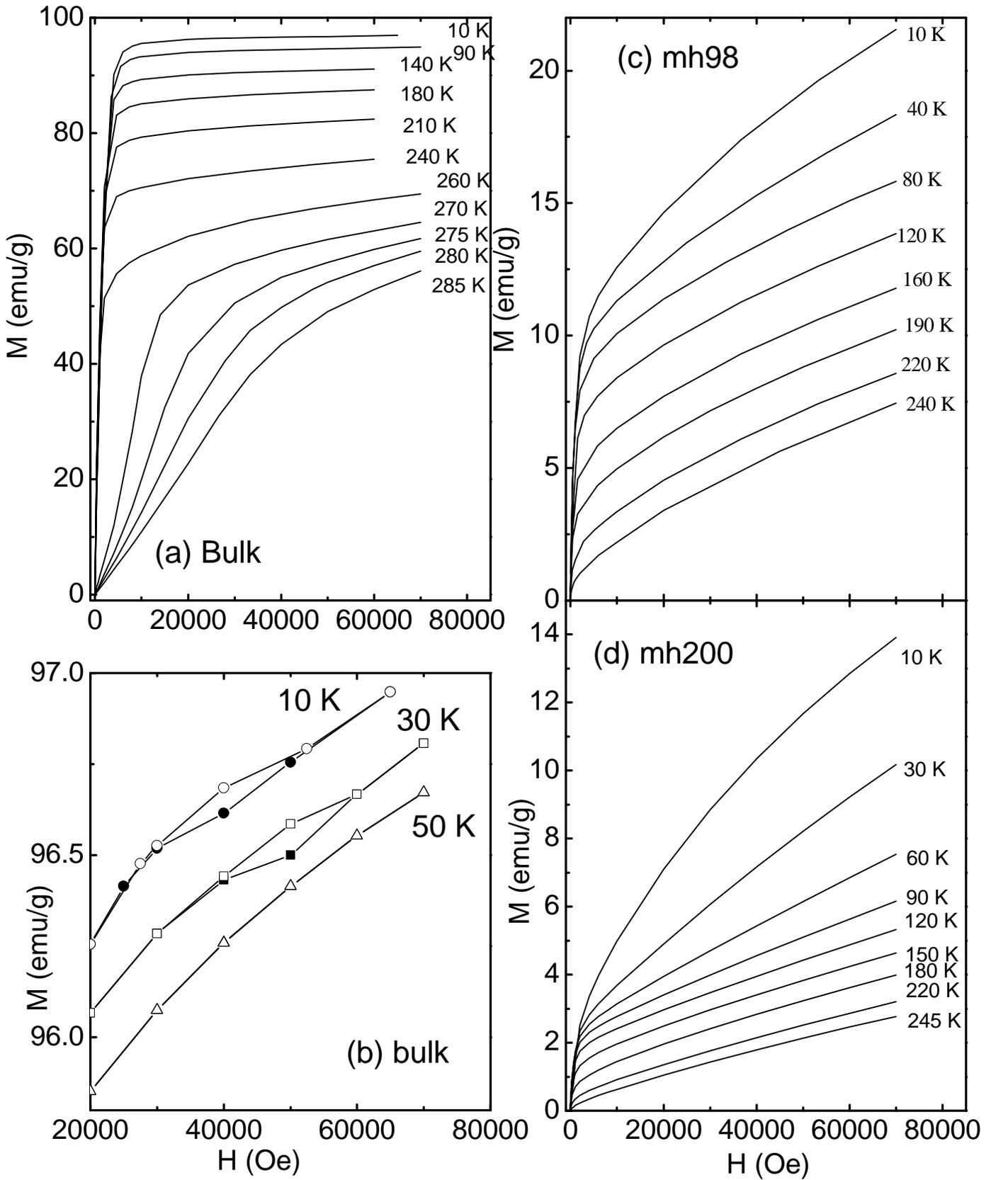
Fig. 8  $M(H)$  data at selected temperatures for (a) bulk, (c) mh98, (d) mh200 samples. The minor loops at higher field (20 kOe-80 kOe) and temperature range 10 K-30 K are shown in (b). Solid and open symbols represent magnetization data during field increase and decrease, respectively.
