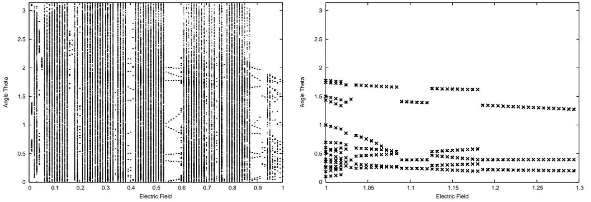
FIG. 9: The upper half of the projection of the multi-furcation diagram onto the  $\theta$  axis, for  $\epsilon$  in the range  $[0.01; 1]$ . The last  $10^3$  points of trajectories with length  $10^7$  collisions have been plotted (left panel). The multi-furcation diagram in the  $(\epsilon; \theta)$  plane, for  $\epsilon$  in the range  $[1, 1.3]$ , from the last  $10^3$  collisions out of a trajectory of  $10^7$  collisions (right panel).
