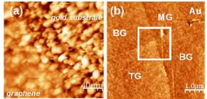
FIG. 2: (color online). (a) The 200 nm x 200 nm STM topography showing gold-graphene interface. (b) The 5444 nm x 5444 nm STM topography showing coexistence of MG, BG and TG flakes. STS measurements were carried out in the surface region denoted by a square.
