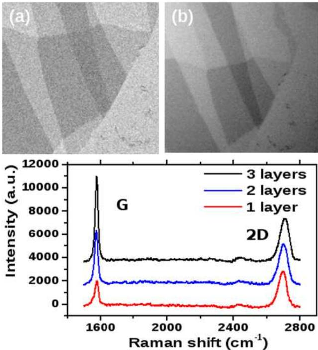
FIG. 1: (color online). (a),(b) OM (left) and SEM (right) images of MG, BG and TG deposited onto Au/Cr/SiO<sub>2</sub>/Si substrate. Typical Raman spectra of MG, BG and TG are presented below.
