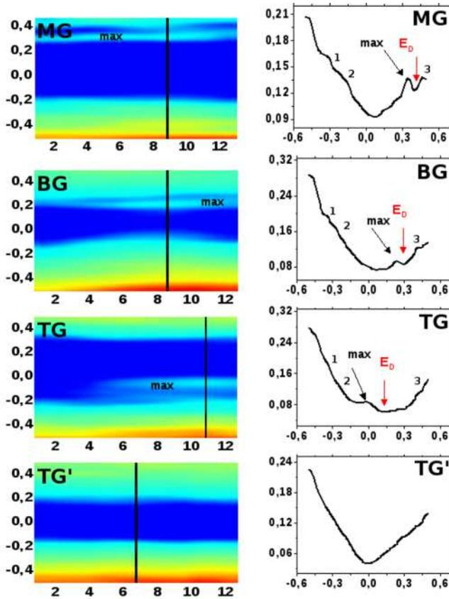
FIG. 4: (color online): blue, green, red - low, intermediate, and high value of  $dI/dV$ , respectively). Left column.  $dI/dV$  ( $E$ , line) maps recorded on MG, BG and TG/TG'. Vertical scale - energy in eV relative to the Fermi level, horizontal scale - length in nanometers. Right column.  $dI/dV$  profiles. Vertical scale  $dI/dV$ , horizontal scale energy in eV relative to the Fermi level
