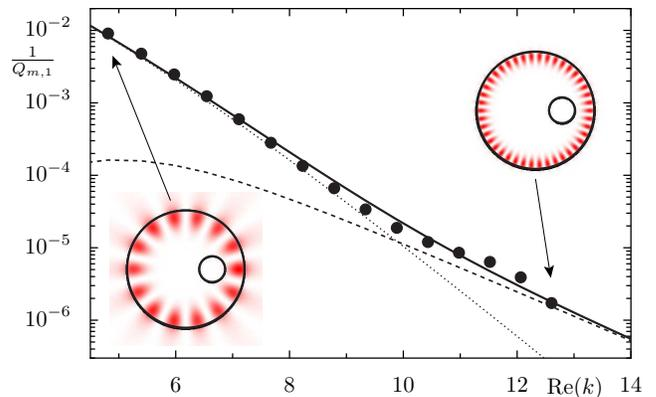
FIG. 3: (Color online) Inverse quality factors  $1/Q$  for the annular microcavity with  $n_{\text{eff}} = 2.0$ . Shown is the theoretical prediction (solid line) which is the sum of the direct tunneling contribution (dotted line) and the dynamical tunneling contribution (dashed line, Eq. (15)), and numerical data (dots) for  $m = 7, \dots, 21$  and  $n = 1$  at  $d = 0.33$ . The insets exemplarily show the resonant states of angular quantum number  $m = 7$  (left) and  $m = 21$  (right).
