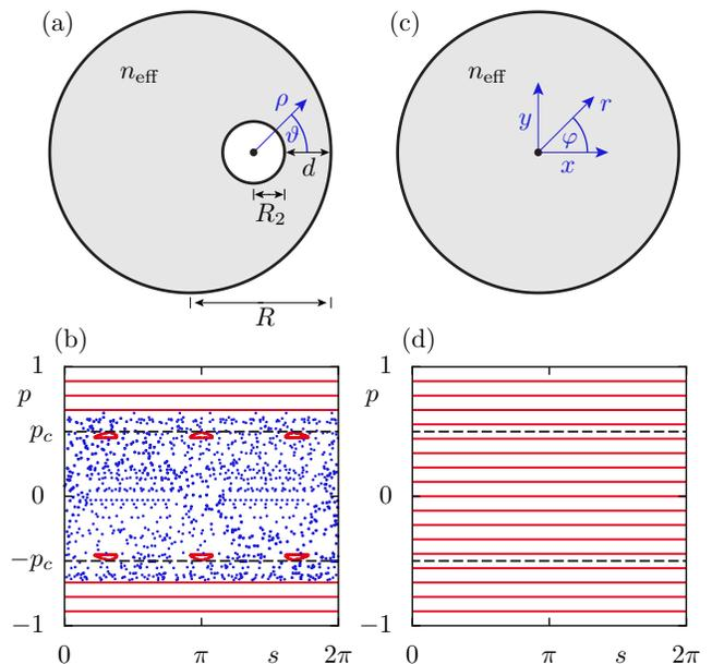
FIG. 2: (Color online) (a) Annular cavity with  $R = 1$ ,  $R_2 = 0.22$ , and  $d = 0.33$ . (b) Corresponding Poincaré section ( $s, p = \sin \chi$ ) for  $n_{\text{eff}} = 2.0$ , where  $s$  is the arclength along the boundary and  $\chi$  is the angle of reflection. Between the critical lines (dashed) with  $|p_c| = 1/n_{\text{eff}}$  is the leaky region, where the condition for total internal reflection is not fulfilled. (c) Circular cavity and (d) its completely regular phase space.
