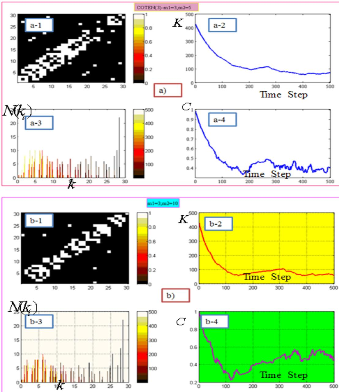
Figure 10. The results of the modified CONA algorithm: a)  $m_1 = 5, m_2 = 3$  and  $\alpha = 1, \beta = 10$  -a<sub>1</sub>: final adjacency matrix over 500 generations, a<sub>2</sub>:  $K$  (number of total edges)-Time step, a<sub>3</sub>: frequency of edges during procedure and a<sub>4</sub>:  $C$  (Clustering Coefficient)-Time Step; b)  $m_1 = 10, m_2 = 3$
