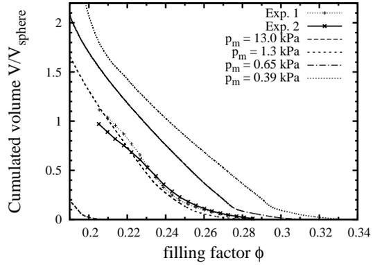
Fig. 15.— Cumulated volume over filling factor. While  $p_m = 13$  kPa, i.e. the unmodified ODC relation, and  $p_m = 0.39$  kPa as well as  $p_m = 0.65$  kPa yield too small and too high compression values, respectively,  $p_m = 1.3$  kPa matches very well for  $\phi \gtrsim 0.22$ . The experimental data are identical to those shown in Fig. 11 (bottom)
