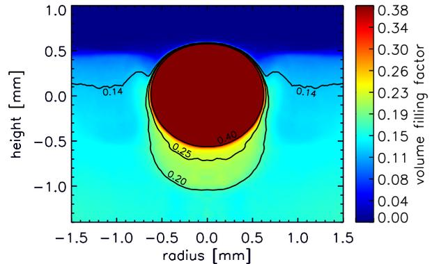
Fig. 9.— Spatial averaged volume filling factors mirrored at the vertical center line. The volume under the sphere is compacted to a volume filling factor  $> 0.2$  (yellow), while the surrounding material is nearly unaffected (light blue).
