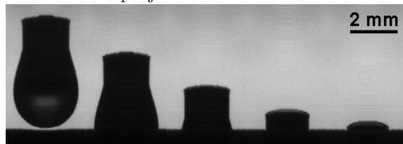
Fig. 4.— Image sequence of a decelerated projectile. The time between two images is 1.7 ms.
