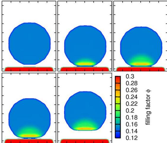
Fig. 19.— Sequence of snapshots of an SPH simulation of a fluffy dust aggregate with a radius of 0.5 mm, impacting a solid target at a velocity of  $0.2 \text{ m s}^{-1}$ . The time differences between subsequent images are 0.35 ms, 0.32 ms, 0.23 ms, and 4.45 ms, respectively. The colors denote different degrees of internal compaction. [See the electronic edition of the *Journal* for accompanying mpeg animations.]
