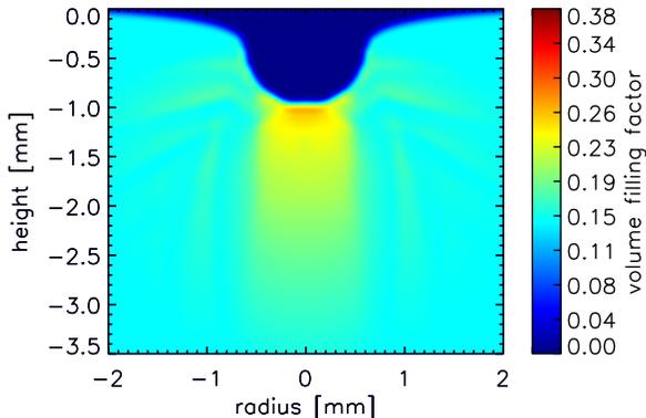
Fig. 16.— Spatially distributed compression as calculated in the SPH simulation with  $Y = \sqrt{\Sigma \cdot |T|}$  and  $p_m = 1.3 \text{ kPa}$ ; same color scale as Fig. 9; the projectile is not plotted. Although the filling factor of compressed material is comparable to the one in the experiments, the compressed volume reaches significantly deeper.
