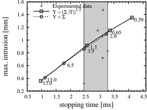
Fig. 13.— Stopping time - intrusion diagram. Experimental data for spheres of 1 mm radius. Labels indicate the  $p_m$  values (in kPa) for the modification of the compressive strength curve. For the  $Y = \Sigma$  model the best match in stopping time and intrusion depth is found for  $p_m = 3.9$  kPa. For the  $Y = \sqrt{\Sigma|T|}$  model the best approximation is given for  $p_m = 1.3$  kPa.
