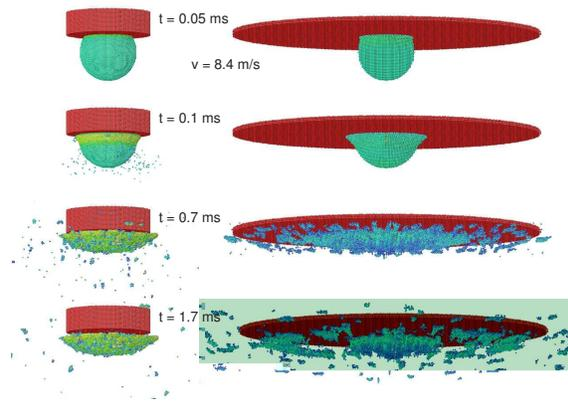
Fig. 21.— Image sequence of an SPH simulation, identical to the experiment shown in Fig. 20. The simulation with the calibrated parameters (**left**) cannot reproduce the experimental results, whereas a simulation using an unidirectional compression curve and  $\Sigma = |T|$  (**right**) can reproduce the qualitative findings of Fig. 20. [See the electronic edition of the Journal for accompanying mpeg animations.]
