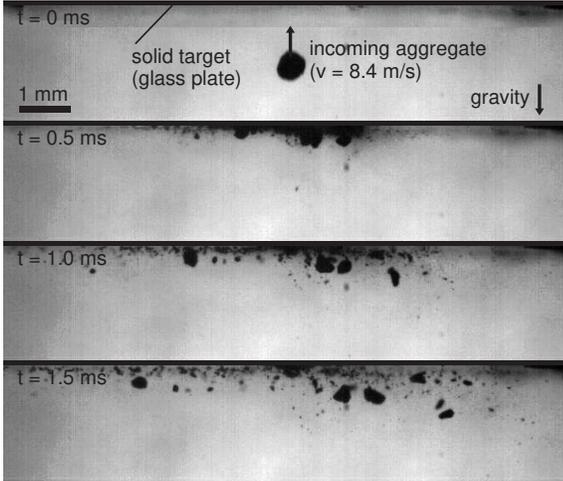
Fig. 20.— Image sequence of an experiment, in which a fluffy dust aggregate impacts a solid target at  $8.4 \text{ m s}^{-1}$ . Part of the aggregate sticks to the target after the collision. [See the electronic edition of the Journal for accompanying mpeg animations.]
