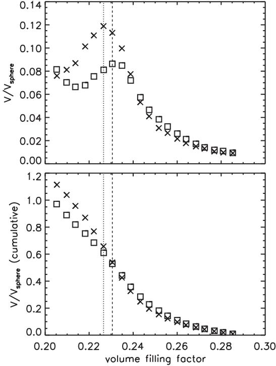
Fig. 11.— **Top:** Distribution of volume filling factors only for the compressed area underneath the impacted sphere for two experiments. The dashed and dotted lines mark the most occurring volume filling factors for each curve, lying at  $\phi \approx 0.23$ . **Bottom:** Normalized volume fraction of compacted area corresponding to a volume filling factor  $> \phi$ .
