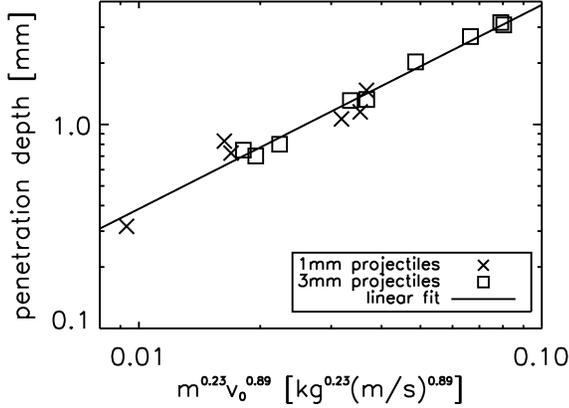
Fig. 6.— The best relation for the penetration depths from a  $\chi^2$  test yields a dependence of  $D \propto m^{0.23} v_0^{0.89}$ . The intuitive relation  $D \propto m v A^{-1}$  is possible within the uncertainties.
