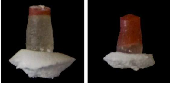
Fig. 7.— Dust sticks to the projectiles after pulling them out of the dust sample. This is an indication of compacted material under the projectile as will be confirmed in Sect. 3.4.
