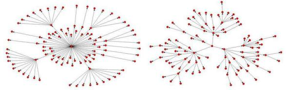
Figure 4: The left tree is a shortest spanning tree created from a scale-free network, which is from BA model with average degree 6. The right one is from a random network with the same average degree as the scale-free network. It clear that the depth of such effective directed trees is related to the topology of the original networks.
