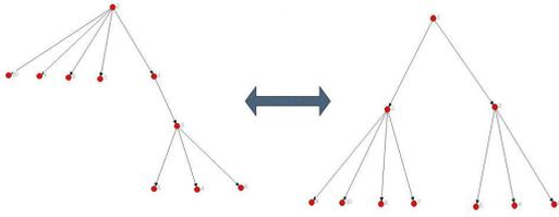
Figure 3: Given a network with 10 nodes, the left tree is created by adopting the node with largest degree as the root, and the right one is the shortest tree based on this topology. Obviously, the center is not simply the node with the largest degree.
