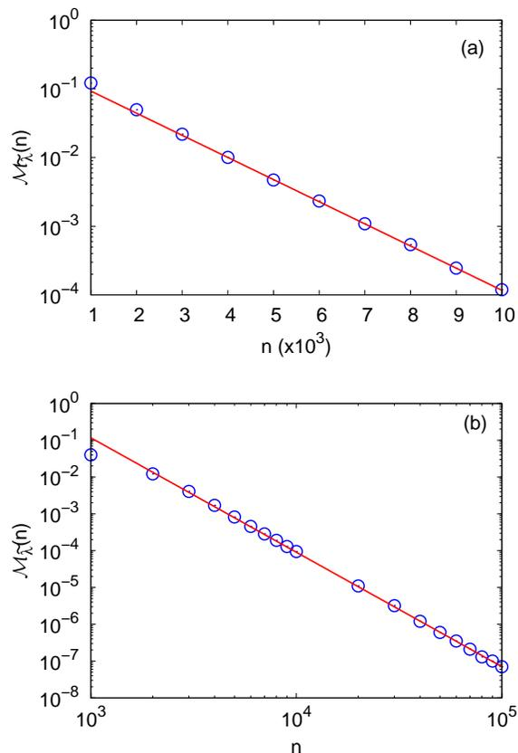
FIG. 4: Decay  $\mathcal{M}_{\bar{\lambda}}(n)$  (symbols) together with a regression fit (full lines) for the map (8) with (a)  $\varepsilon = 0.5$  and  $\gamma = 1$  (exponential rate decay  $0.87 \pm 0.01$ ) and (b)  $\varepsilon = 0$  and  $\gamma = 1$  (polynomial rate decay  $3.05 \pm 0.05$ ). Both fits were done by starting at  $n = 3000$ .
