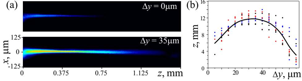
Fig. 2. (a, [Media 1](#)) Experimentally recorded images of the light scattered from a single nematicon at different positions  $\Delta y$  in the cell relative to the upper plate; the input beam power is 4.7 mW. (b) Averaged distance (solid line) at which the intensity of the scattered radiation is at its half-maximum; data points are shown by colored dots in black for a single nematicon, in red for two in-phase and in blue for two out-of-phase nematicons.
