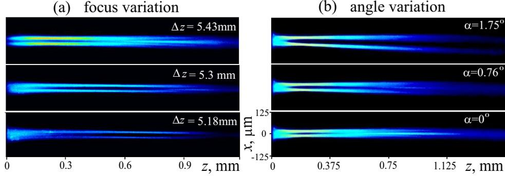
Fig. 4. Experimental results on the interaction between two nematicons. (a, [Media 4](#)) Effects due to varying the  $z$ -position of the focal plane of the input objective lens (5.5 mm) with respect to the input facet; here  $\Delta z$  is the distance between the objective and the NLC cell. (b, [Media 5](#)) Effects due to variations in the launch angle  $\alpha$  between two in-phase nematicons.
