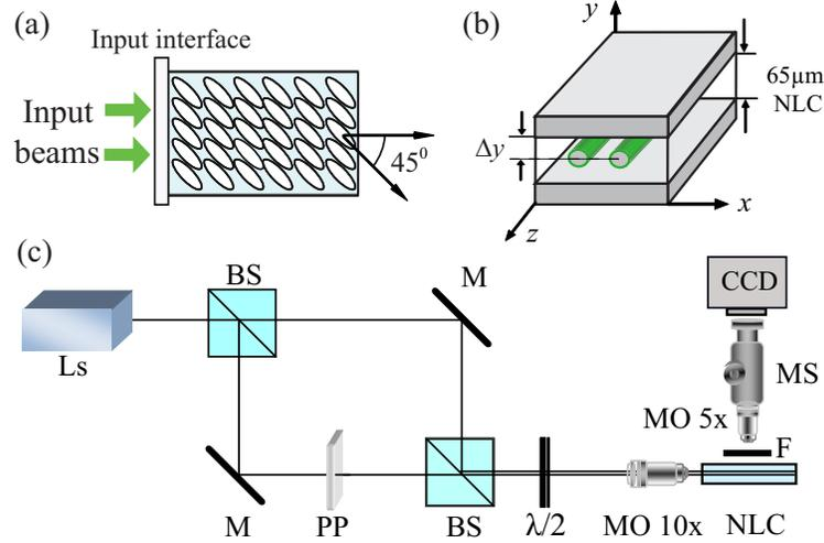
Fig. 1. (a) Top view of the NLC planar cell. The ellipses indicate the orientation of the molecules in the plane  $(y, z)$ . (b) Perspective view of the NLC cell with two nematons. (c) Experimental setup: Ls – cw-laser ( $\lambda = 532\text{nm}$ ), BS – beam splitters, PP – parallel face plate for adjusting the phase difference, M – mirrors,  $\lambda/2$  – half wavelength plate, MO – microscope objectives, NLC – nematic liquid crystal cell, F – filter, MS – microscope, CCD – camera.
