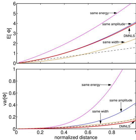
FIG. 1: (Color online) Mean (top) and variance (bottom) of the soliton phase as reconstructed with standard MC simulations. Thick red lines: DMNLS; blue lines: constant-dispersion NLSE soliton with same amplitude as the DMS; magenta lines: NLSE soliton with same energy; orange lines: NLSE soliton with same width. The dashed black lines show the predictions from perturbation theory.
