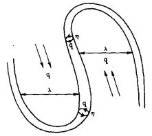
Fig. 7: Tennekes' simple model for the small scale structure of turbulence [15] (reprinted with permission of the AIP).
