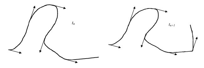
Fig. 2: turning the continuous cascade of bending events into a discrete one. A bending event is defined by the appearance of a new quasi-cusp on the vortex line: the angle between two successive tangent vectors to the line is equal to a given number (for instance  $\pi/2$  in the considered case)
