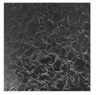
Fig. 3: Wrinkling of a fluid surface in isotropic turbulence: Karweit, John Hopkins Univ. 1968 [21]. Here, material lines are stretched, but a clear analogy with vortex tubes can be made, since they can be considered as materially linked to the fluid [16]. (reprinted with permission of the author).
