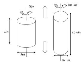
Fig. 1: axial stretching of a portion of a vortex tube
