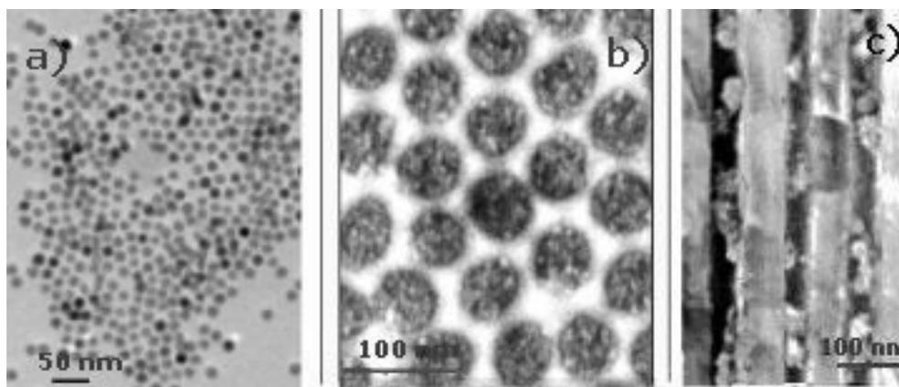
Fig. 1. a) TEM of the nanoparticles; b) and c) FESEM of the membrane channels with nanoparticles: b) view from the top; c) view from the edge
