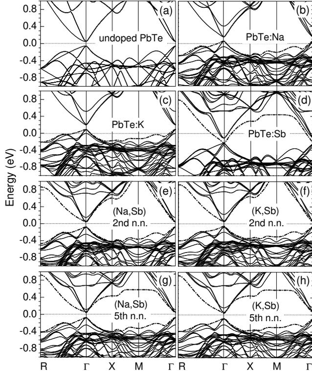
FIG. 10: Band structures of undoped PbTe and PbTe doped with Na, K, Sb, (Na,Sb), and (K,Sb). The impurity-induced bands are represented by the dash-dotted curves. The results were obtained in calculations using the  $(2 \times 2 \times 2)$  supercell with SOI included. The two impurity atoms in a pair are either the second (2nd n.n.) or fifth (5th n.n.) nearest neighbors of one another. The Fermi level (0 eV) is set to the highest occupied states or in the band gap.
