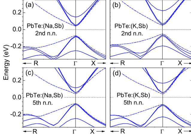
FIG. 11: (Color online) Band structures of PbTe doped with (Na,Sb) and (K,Bi) impurity pairs showing the arrangement of the energy bands near the  $\Gamma$  point. The impurity-induced bands are represented by the dash-dotted curves. The Fermi level (0 eV) is in the band gap.
