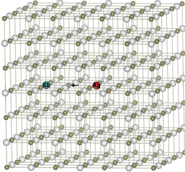
FIG. 4: (Color online) Relaxed structure of (Ag,Sb)-doped PbTe where the two impurity atoms are the second nearest neighbors of one another in a  $(3\times 3\times 3)$  supercell. Large spheres are Ag (red) and Sb (blue), medium (gray) spheres Pb, and small (dark gray) spheres Te. The Te atom (marked by the arrow) in the Ag-Te-Sb chain is shifted towards Sb by  $\sim 0.3$  Å, resulting in different Ag-Te and Sb-Te bond lengths.
