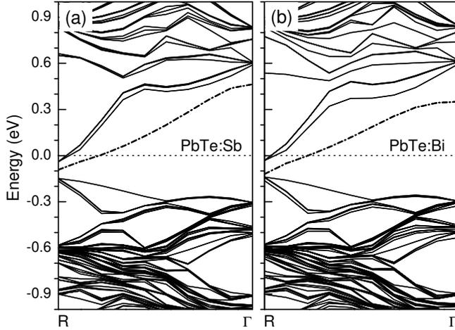
FIG. 7: Band structures of PbTe doped with (a) Sb and (b) Bi obtained in calculations using  $(3\times 3\times 3)$  supercells with SOI included. The impurity-induced bands are represented by the dash-dotted curves. Note that the zero of the energy may not be given accurately because the calculations scanned only a very small part of the BZ.
