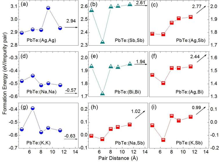
FIG. 1: (Color online) Formation energies of various impurity pairs in PbTe as a function of the pair distance. The results were obtained in calculations using  $(2 \times 2 \times 2)$  supercells; SOI was not included (see the text). The values given with the arrows are the formation energies of the pairs at infinite pair distance (obtained by adding up the formation energies of the isolated impurities).
