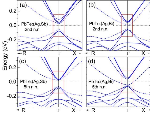
FIG. 9: (Color online) Band structures of PbTe doped with (Ag,Sb) and (Ag,Bi) impurity pairs showing the differences in the band gap and in the arrangement of the energy bands near the  $\Gamma$  point. The impurity-induced bands are represented by the dash-dotted curves. The Fermi level (0 eV) is set to the highest occupied states or in the band gap.
