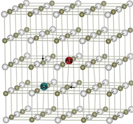
FIG. 3: (Color online) Relaxed structure of (Ag,Sb)-doped PbTe where the two impurity atoms are the first nearest neighbors of one another in a  $(2 \times 2 \times 2)$  supercell. Large spheres are Ag (red) and Sb (blue), medium (gray) spheres Pb, and small (dark gray) spheres Te. The two Te atoms (marked by the arrows) in between Ag and Sb are shifted towards Sb by  $\sim 0.2$  Å, resulting in different Ag-Te and Sb-Te bond lengths; see Table I.
