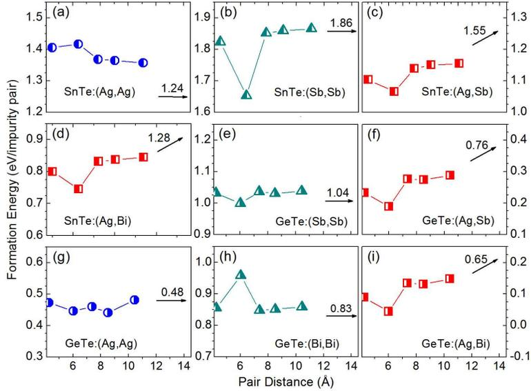
FIG. 2: (Color online) Formation energy of various impurity pairs in SnTe and GeTe as a function of pair distance. The results were obtained in calculations using  $(2 \times 2 \times 2)$  supercells; SOI was not included (see the text). The values given with the arrows are the formation energies of the pairs at infinite pair distance (obtained by adding up the formation energies of the isolated impurities).
