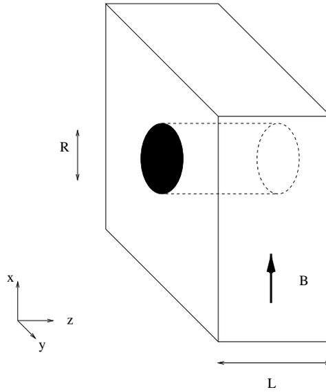
FIG. 1: Schematic view of the experimental setup. The experiment measures the noise of spin magnetization in the  $z$  direction in the presence of an applied constant magnetic field in the  $x$  direction that splits the two spin energy levels by the Larmor frequency  $\omega_L$ . The system has thickness  $L$  in the  $z$  direction, and is extended in the  $x$ - $y$  direction. Noise in the part of the system with transverse size  $R$  and cross section  $A = R^2$  is probed.
