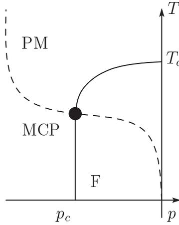
Figure 1. A typical phase diagram of the  $J$  Ising model in two dimensions. The multicritical point (MCP) is described by a black dot and the Nishimori line is drawn dashed.
