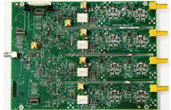
Fig. 11. The analog board realizing four sampling channels. It consists of three stages: splitting the analog input, mixing with four input periodic waveforms (connectors on the rear), and lowpass filtering.
