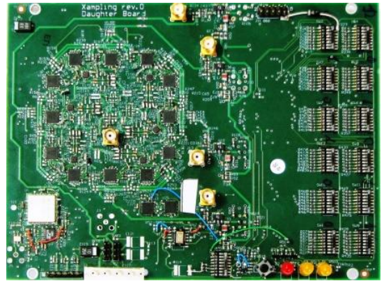
Fig. 15. The digital board provides four sign-alternating periodic waveforms, which are derived from a single SR chain.
