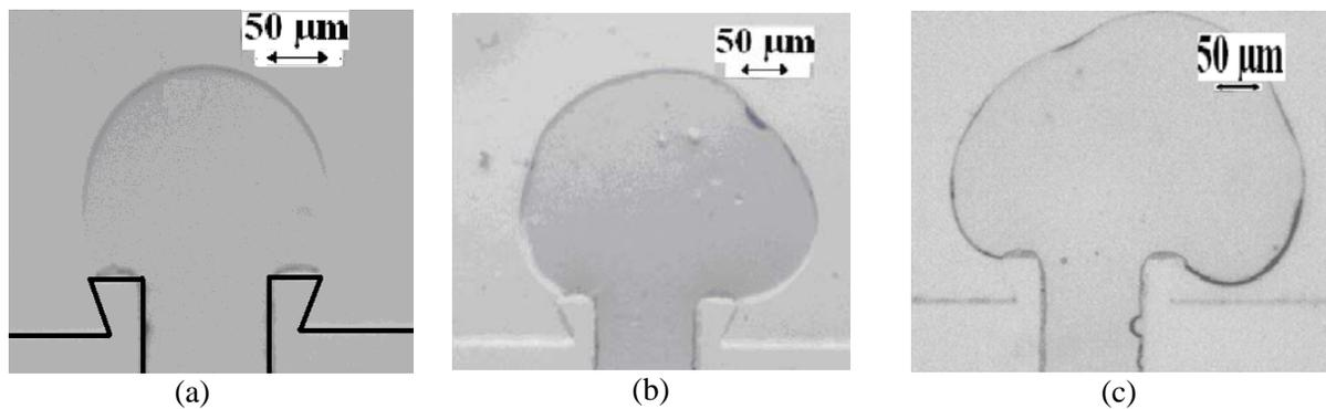
**Figure 5: Microgeometry with overhang. Sequence (a-c) shows and excellent pinning of the contact line.  $\Delta S$  in this case is  $0.021 \text{ mm}^2$ .**
