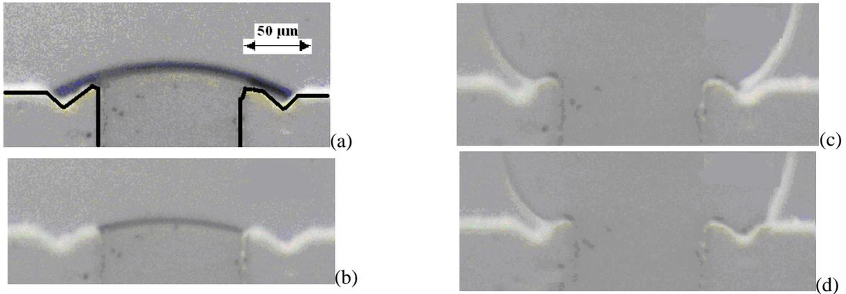
**Figure 3: Microgeometry with pits at the entry of channel D into chamber E. Sequences (a-b) and (c-d) show that the meniscus contact line is not pinned by the pits, when the meniscus shrinks and grows respectively.  $\Delta S$  in this case is  $0 \text{ mm}^2$ .**
