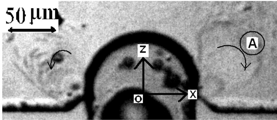
Figure 14: Two microstreaming vortices visible at the left and right of the meniscus vicinity. The excitation frequency is 110V and the voltage is 90 V. Arrows indicate the direction of rotation.
