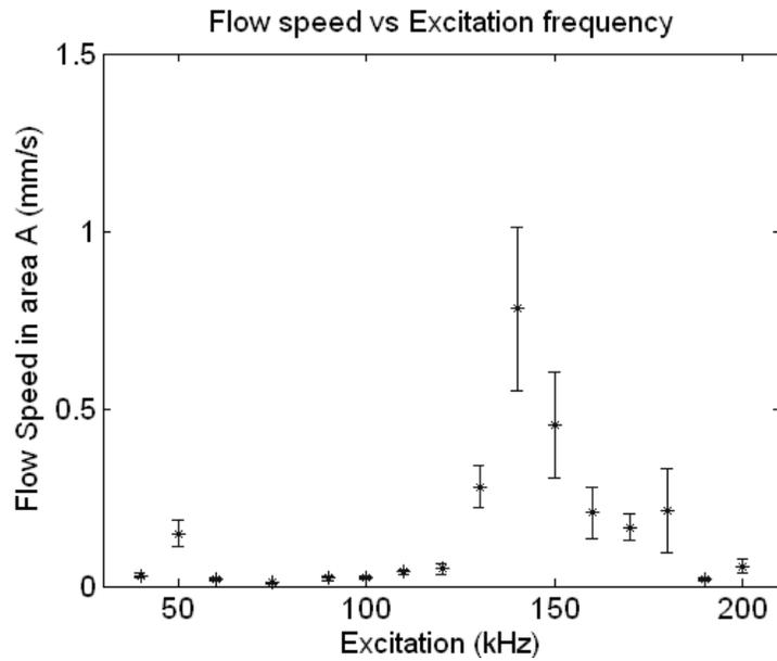
Figure 15: Flow speed in area A (Figure 16) vs excitation frequencies.
