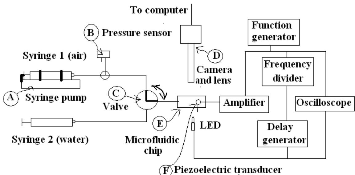
**Figure 2: The experimental setup involves: a microfluidic platform, a piezoelectric actuation system and a visualization system, During the experiment, we connect the valve C to syringe 2, so that water is infused into the system. Then, the valve is shifted to syringe 1 to add a controlled flow rate of air into the system and forms a meniscus.**
