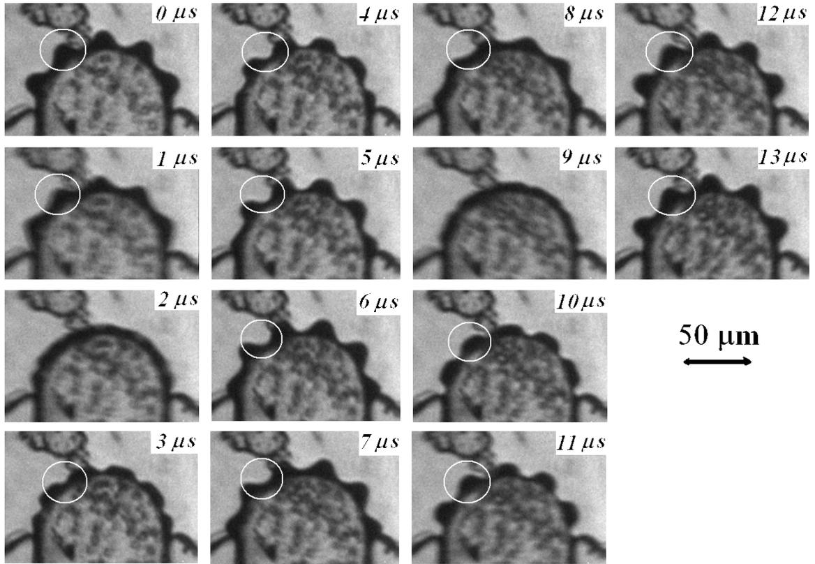
Figure 12: Standing wave on meniscus interface at 150 kHz of excitation, the standing wave is oscillating at 75 kHz. Note that there are drops generated in the air, which are found more often in the standing wave case than the traveling wave case.
