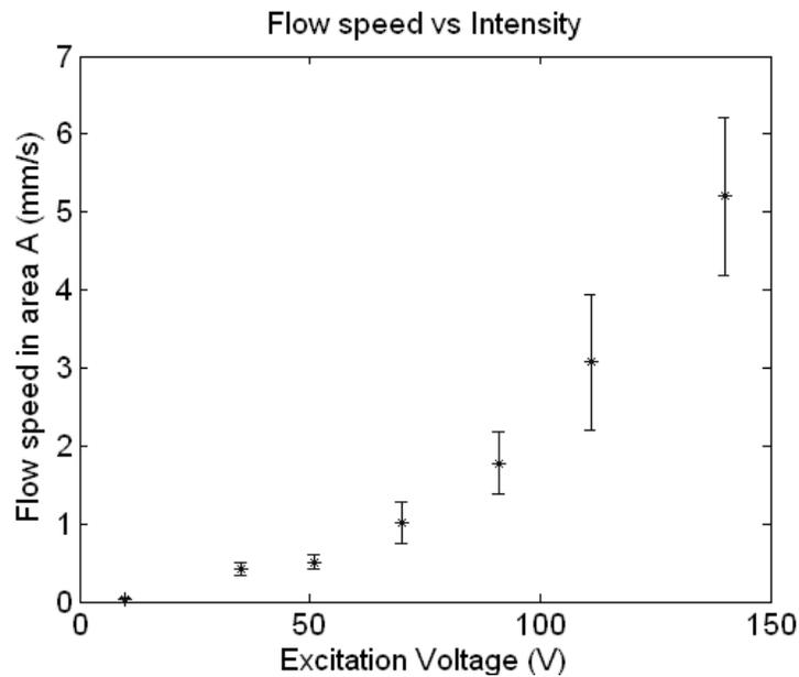
Figure 16: Flow speed in area A of Figure 16 vs intensity of the piezoelectric excitation. The excitation frequency is 100 kHz
