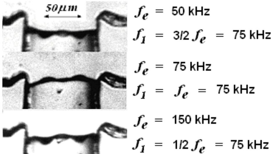
Figure 13: Standing waves at different frequencies.
