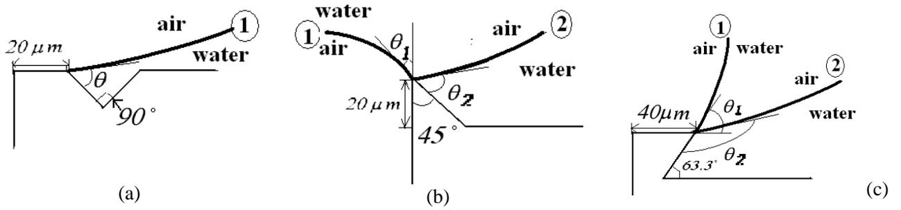
Figure 6: Theoretical analysis for the contact line stable range during bubble growth.
