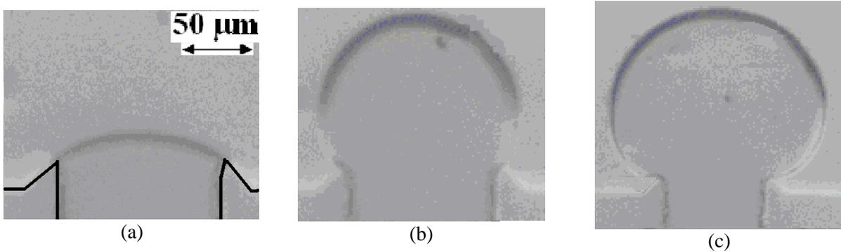
**Figure 4: Microgeometry with peaks at the chamber entry. Sequence (a-c) show how the meniscus contact line is pinned at the peaks.  $\Delta S$  in this case is  $0.011 \text{ mm}^2$ .**
