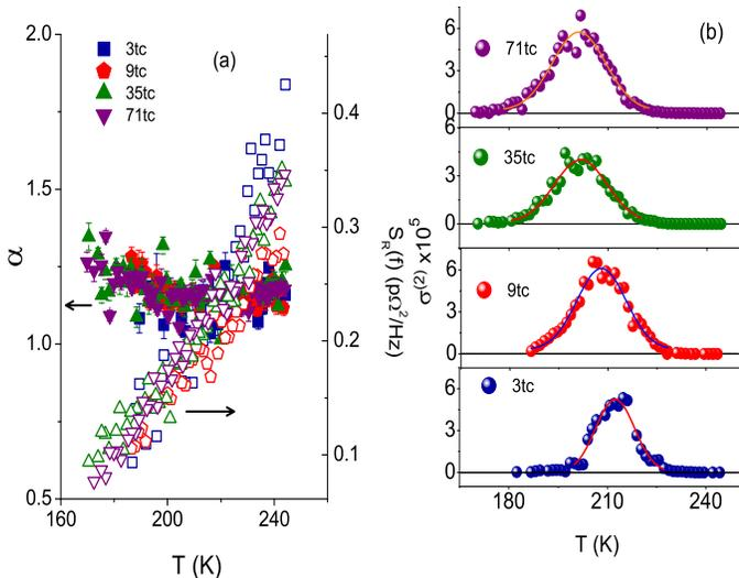
FIG. 6: (Color Online)(a) Power spectral density (open symbols) and the frequency exponent  $\alpha$  (closed symbols) as a function of temperature for various thermal cycles. (b) The variation of  $\sigma^{(2)}$  as a function of temperature for different thermal cycles. The Gaussian expectation is plotted as dotted lines. The deviation from the Gaussian behavior of the second spectrum around the critical temperature is evident. The fits shown are Gaussian.
