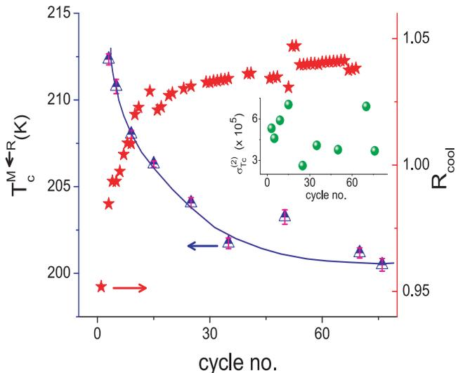
FIG. 7: (Color Online) The variation of  $T_c$  as a function of thermal cycles calculated from the Gaussian fits shown in Fig.6(b). The curve is a guide to the eye. The resistance value at 245K during cooling for the various thermal cycles is also plotted for comparison. The inset shows the variation of  $\sigma^{(2)}$  at  $T_c$  for the various cycles.
