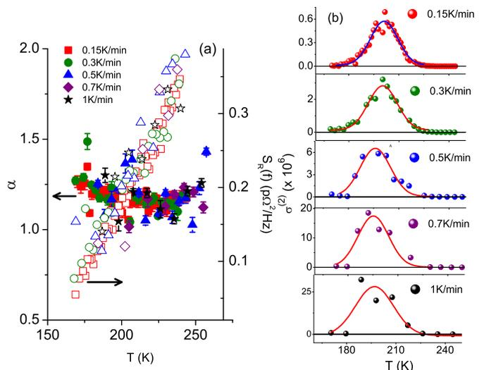
FIG. 8: (Color Online)(a) Power spectral density (open symbols) and the frequency exponent  $\alpha$  (closed symbols) as a function of temperature for various drive rates. (b) The variation of  $\sigma^{(2)}$  as a function of temperature for the various drive rates. The Gaussian expectation is plotted as dotted lines. The deviation from the Gaussian behavior of the second spectrum around the critical temperature is evident. The fits shown are Gaussian.
