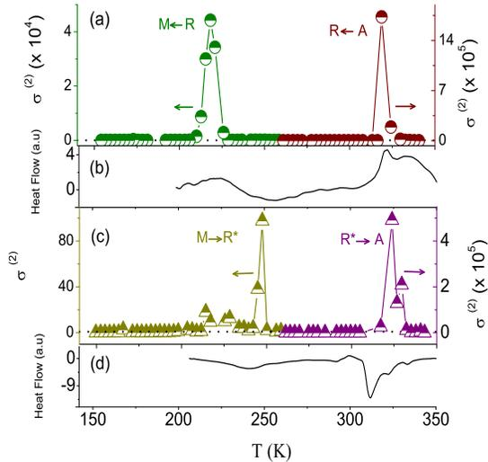
FIG. 4: (Color Online) The integrated value of the normalized second spectra  $\sigma^{(2)}$  as a function of temperature showing the peaks corresponding to the transitions for (a) cooling and (c) heating. The corresponding DSC plots are shown in the lower panels (b) and (d). The calculated Gaussian value integrated over the frequency bandpass is shown as a dotted line. The details about the transforming phases are denoted in (a) and (c).
