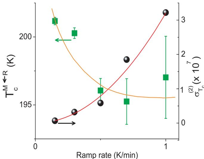
FIG. 9: (Color Online) The critical point  $T_c$  calculated from the Gaussian fits in Fig.8(b), as a function of drive rate. The magnitude of  $\sigma^{(2)}$  at  $T_c$  as a function of drive rate is plotted on the right hand side axis. The curves are guide to the eye.
