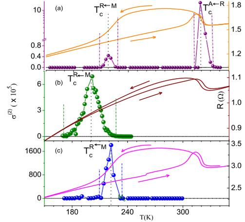
FIG. 5: (Color Online) Integrated value of the normalized second spectra  $\sigma^{(2)}$  as a function of temperature for three different samples shown along with the corresponding resistance plots. The heating and cooling directions are shown using appropriate arrows. The region over which  $\sigma^{(2)}$  deviates from the Gaussian background (dotted line) is marked using vertical lines. The point at which  $\sigma^{(2)}$  reaches its maximum is defined as the critical temperature  $T_c$ .
