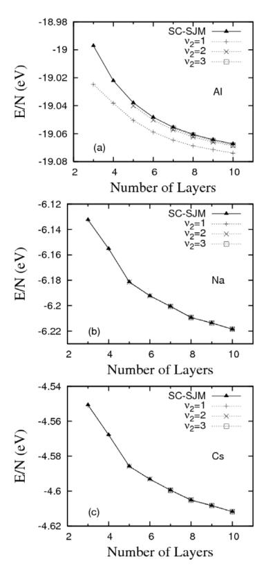
**Figure 4.** (a)-Total energies of Al slabs in the SC-ISJM as functions of the number of layers, V, for different surface parameters,  $V_2$ . For comparison, we have also included the SC-SJM results. Similarly, (b) and (c) correspond to Na and Cs slabs. As is seen, the overlapping data points in Na and Cs cases imply that the interaction energy between the electrons and the ions are not sensitive to the exact positions of the ions.
