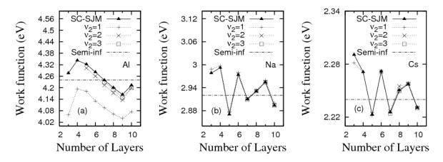
**Figure 6.** (a)-Work functions of Al slabs in the SC-ISJM as functions of the number of layers,  $\nu$ , for different surface parameters,  $\nu_2$ . The  $\nu_2 = 1$  plot corresponds to the equilibrium state. For comparison, the SC-SJM and semi-infinite jellium [15, 16] results are included. Similarly, (b) and (c) correspond to Na and Cs slabs.
