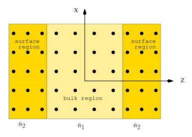
Figure 2. Schematic representation of the simplified ISJM for a slab with three main regions. The system is extended to infinity in the x and y directions. In this example, each surface region contains three atomic layers, while the inner bulk region contains four atomic layers. The interlayer spacings in the surface region can be different from that in the inner region.
