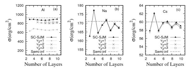
**Figure 7.** (a)-Surface energies of Al slabs in the SC-ISJM as functions of the number of layers,  $\nu$ , for different surface parameters,  $\nu_2$ . The  $\nu_2 = 1$  plot corresponds to the equilibrium state. For comparison, the SC-SJM and semi-infinite jellium [15, 16] results are included. Similarly, (b) and (c) correspond to Na and Cs slabs.
