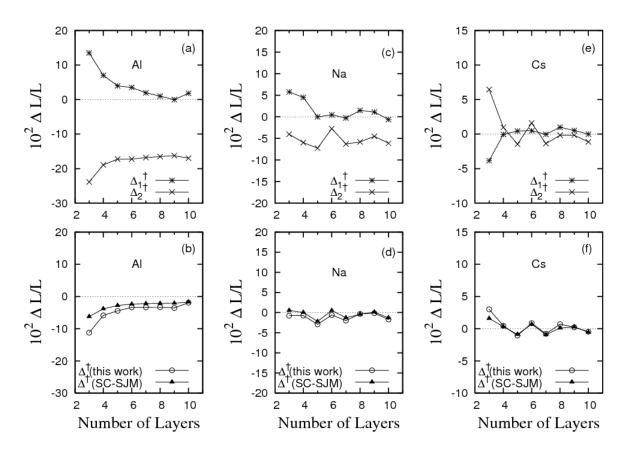
**Figure 5.** (a) Surface and bulk relaxations of Al slabs in their equilibrium states as functions of the number of atomic layers,  $\nu$ . (b) The overall relaxations of Al slabs in the SC-ISJM and SC-SJM as functions of  $\nu$ . Similarly, (c)-(d) correspond to Na slabs, and (e)-(f) correspond to Cs slabs.
