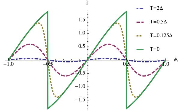
**Figure 2.** Persistent current  $I$  (measured in units  $e\Delta/2\pi$ ) as a function of the magnetic flux  $\phi_x$  for  $\kappa = 3$  at different temperatures:  $T = 0$ ,  $T = 0.125\Delta$ ,  $T = 0.5\Delta$  and  $T = 2\Delta$ .
