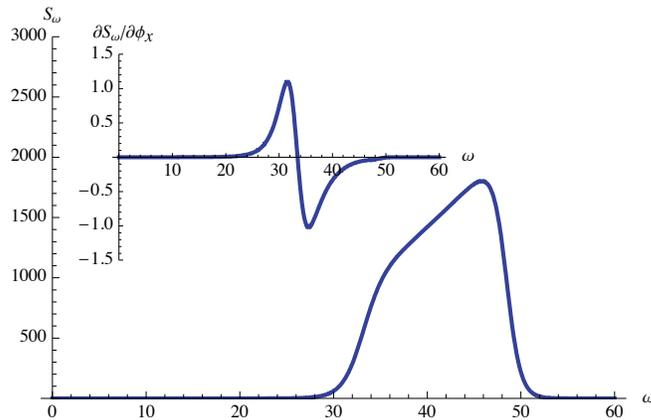
**Figure 3.** Zero temperature PC noise spectrum  $S_\omega$  (arbitrary units) and its derivative with respect to the flux  $\partial S_\omega / \partial \phi$  (arbitrary units) as functions of  $\omega$  (measured in units of  $1/2MR^2$ ) for an ensemble of rings (or for a ring containing many independent channels) with  $U_0$  uniformly distributed within the interval from  $30/MR^2$  to  $65/MR^2$ .
