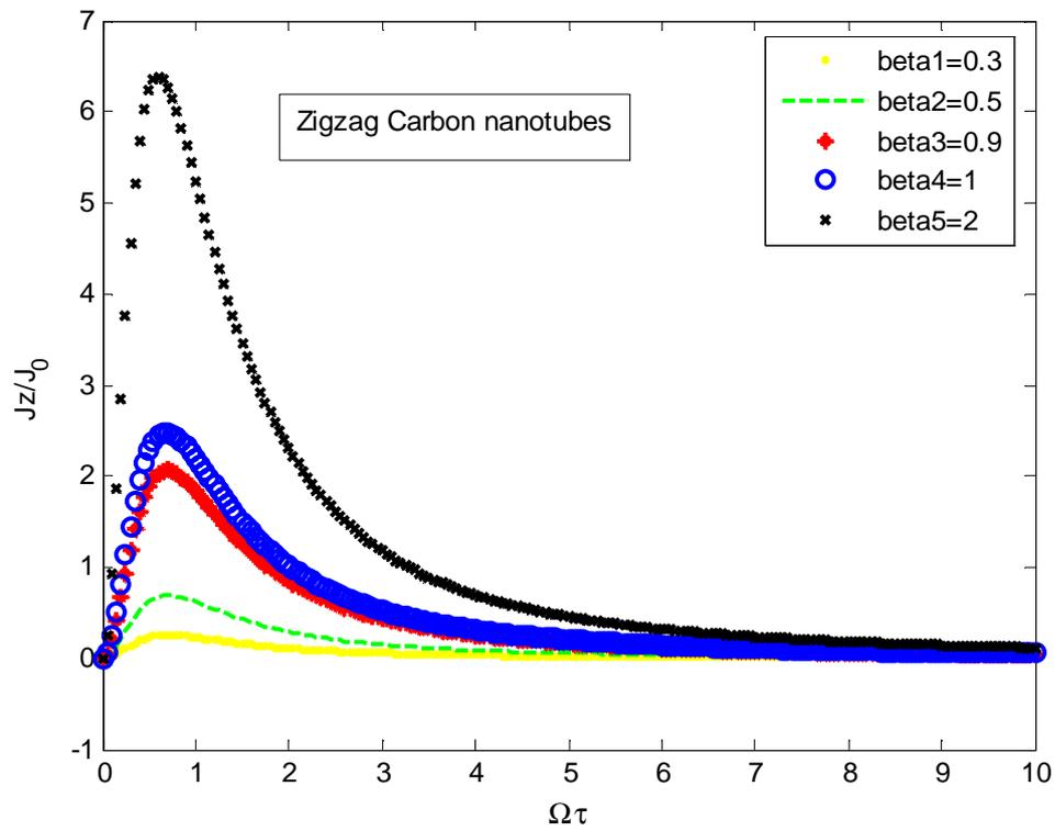
**Fig. 3.**  $J_z/J_0$  is plotted against  $z\tau = \Omega\tau$  for  $(\text{---}\cdot\text{---}) \beta_1 = 0.3$ ;  $(\text{---}\cdot\text{---}) \beta_1 = 0.5$ ;  $(\text{---}\cdot\text{---}) \beta_1 = 0.9$ ;  $(\text{---}\cdot\text{---}) \beta_1 = 1$ ;  $(\text{---}\cdot\text{---}) \beta_1 = 2$ .
