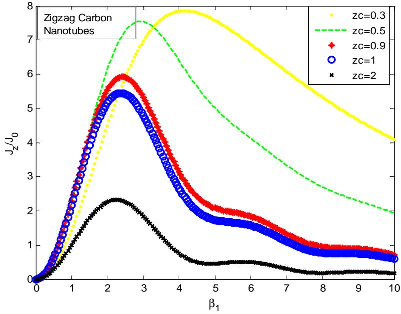
**Fig. 5.**  $J_z/J_0$  is plotted against  $\beta_1$  for (---)  $zc = \Omega\tau = 0.3$ ; (---)  $zc = \Omega\tau = 0.5$ ; (\*\*\*)  $zc = \Omega\tau = 0.9$  (ooo)  $zc = \Omega\tau = 1$ ; (---)  $zc = \Omega\tau = 2$ . When the phase shift  $\varphi$  lies between  $\frac{\pi}{2}$  and  $\frac{3\pi}{2}$
