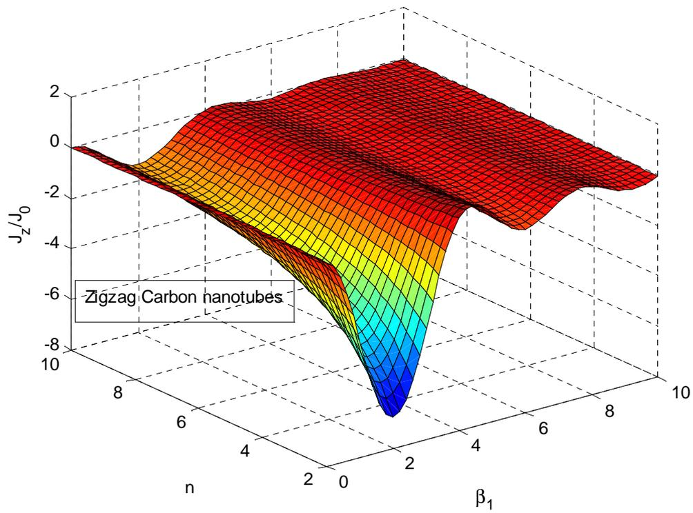
**Fig.4.**  $J_z/J_0$  is plotted against  $\beta_1$  for Zigzag Carbon nanotubes.
