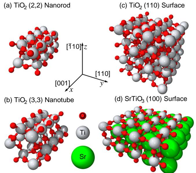
FIG. 1: Structural schematics for (a) TiO<sub>2</sub> (2,2) nanorod, (b) TiO<sub>2</sub> (3,3) nanotube, (c) TiO<sub>2</sub> (110) surface and (d) SrTiO<sub>3</sub> (100) TiO<sub>2</sub> and SrO terminated surfaces. Axes and Miller indices for the rutile structures are shown for (a) and (c).
