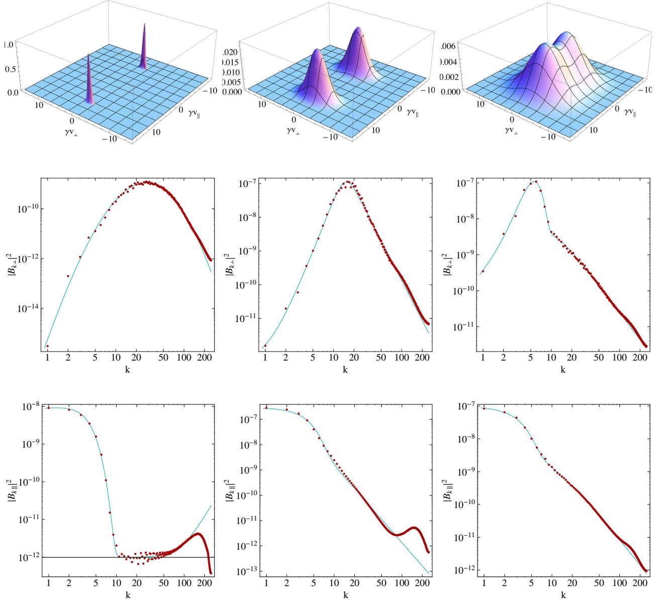
FIG. 9.— A representative sample of snapshots of (top to bottom) the particle distribution,  $F(\gamma v_{\perp}, \gamma v_{\parallel})$ , the perpendicular,  $|B_{k\perp}|^2$ , and parallel,  $|B_{k\parallel}|^2$ , magnetic field spectra before, at and after saturation (left to right:  $t = 6, 10, 30$ ) for the 3D PIC simulation with  $\Gamma = 10$ . The blue curves are the empirical models, while the red dots are computed directly from the data.
