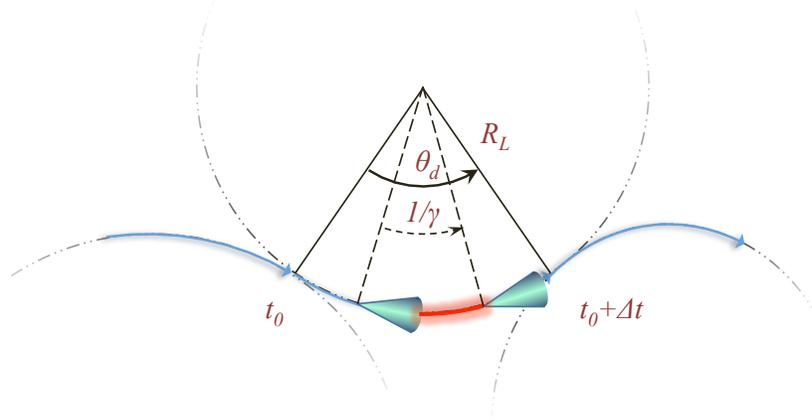
FIG. 5.— Cartoon showing the piecewise circular decomposition of a particle trajectory. For each segment of a certain curvature (Larmor) radius,  $R_L$ , and the deflection angle,  $\theta_d$ , radiation is produced at times between  $t_0$  and  $t_0 + \Delta t$ . Radiation is beamed directly toward an observer on the right within a highlighted  $\sim 1/\gamma$  part of the segment.
