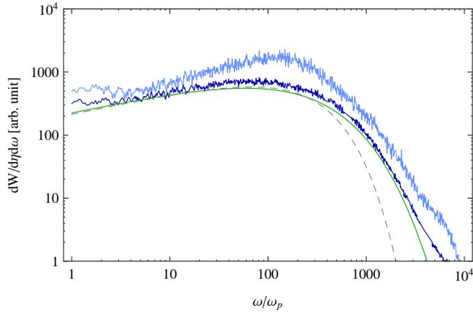
FIG. 12.— The PIC spectrum from the ‘frozen field’ simulation (dark blue) and the original spectrum from Fig. 10(left) (light blue) are shown (in both,  $\Gamma = 10$ ). The magnetic field structure is nearly identical in both, but the trapped population is practically absent in the ‘frozen-field’ case. The corresponding synchrotron spectrum for the actual particle distribution (green) and for the monoenergetic electrons (dashed grey) are also shown for comparison.
