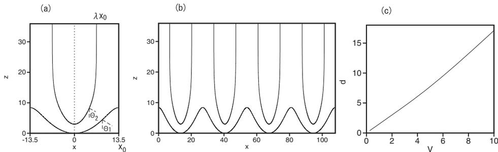
FIG. 3: (a) A single pore solution at  $\lambda = 0.5, x_0 = 13.5, V = 2$  and  $b_1/a = 0.5$ . (b) An array of pore structures. (c) Thickness  $d$  as a function of  $V$  for  $\lambda = 0.5, x_0 = 13.5$  and  $b_1/a = 0.5$
