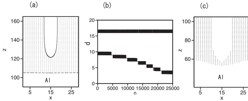
FIG. 4: (a) Pore structure at  $a = 0.042, b_0 = b_2 = g = 0, b_1 = 0.01$  and  $V = 5$  starting from  $d(0) = 16$ . The system size is  $35 \times 400$ . The shaded region represents oxide. (b) Time evolution of the thickness  $d(t)$ . (c) Pore structure at  $a = 0.042, b_0 = b_2 = g = 0, b_1 = 0.01$  and  $V = 5$  starting from  $d(0) = 10$
