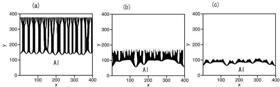
FIG. 7: (a) Pore structure at  $a = 0.02, \alpha_0 = 0.01, k_d = 0, \beta_0 = 0.01, k_o = -1$  and  $V = 2$ . (b) Pore structure at  $a = 0.045, \alpha_0 = 0.05, k_d = 0.2, \beta_0 = 0.0498, k_o = 0$  and  $V = 3$ . (c) Pore structure at  $a = 0.045, \alpha_0 = 0.01, k_d = 1.2, \beta_0 = 0.005, k_o = 1.1$  and  $V = 3$ . Pore structure at  $a = 0.02, \alpha_0 = 0.01, k_d = 0, \beta_0 = 0.01, k_o = -1$  and  $V = 2$ .
