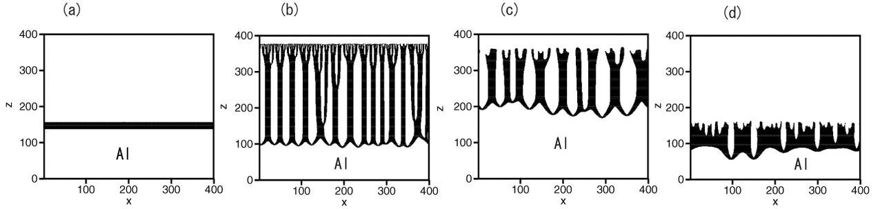
FIG. 6: (a) Flat pattern at  $b_0 = 0, a = 0.015, b_1 = 0.035, b_2 = 0.04, g = 0.0003$  and  $V = 12$ . (b) Pore structure at  $a = 0.02, b_0 = 0, b_1 = 0.01, b_2 = 0.005, g = 0$  and  $V = 2$ . (c) Pore structure at  $a = 0.02, b_0 = 0, b_1 = 0.01, b_2 = 0.005, g = 0.005$  and  $V = 2$ . (d) Pore structure at  $a = 0.045, b_0 = 0.0002, b_1 = 0.01, b_2 = 0, g = 0$  and  $V = 3$ .
