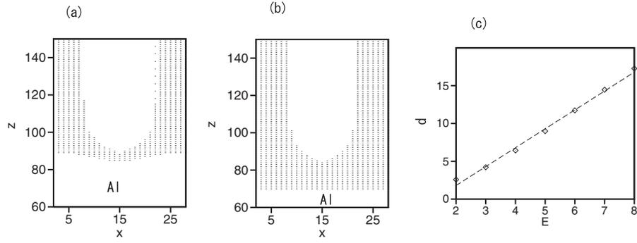
FIG. 5: (a) (b) Pore structures at (a)  $V = 3$  and (b) 7 for  $a = 0.02, b_0 = g = 0, b_1 = 0.01$  and  $b_2 = 0.005$ . (c) Relation of the thickness  $d$  and  $V$ . The dashed line is a linear fitting line.
