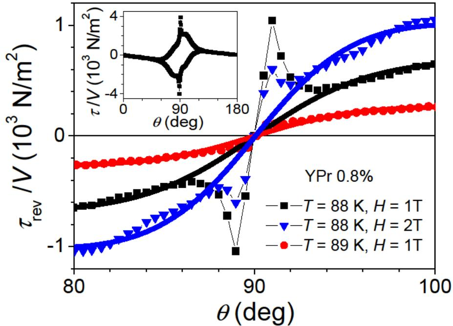
Fig. 6. Angular dependence of the reversible torque for YPr 0.8% at two different temperatures and fields, obtained by averaging the irreversible torque dependence upon clockwise and counterclockwise rotating the sample, indicating deviations from the dependence according to Eq. (1) (represented by straight lines). Inset: Example of the angular dependence of the irreversible torque with pronounced intrinsic pinning close to the  $ab$ -plane.
