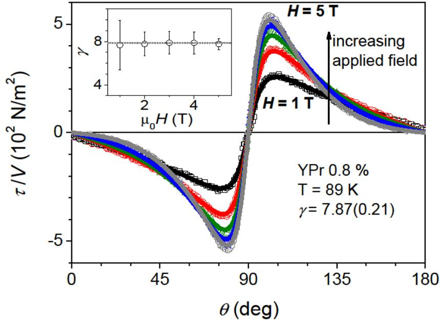
Fig. 5. Angular dependence of the reversible torque for YPr 0.8% at applied magnetic fields between 1 and 5 T at  $T = 89$  K and the corresponding fit of equation (1) to the data. Inset: Field dependence of the anisotropy parameter with maximal errors due to torque hysteresis. The line is a guide to the eye.
