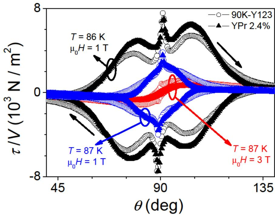
Fig. 7. Angular dependence of the irreversible torque for two crystals with the same oxygen content; open symbols: 90K-Y123, full symbols: YPr 2.4%. The torque maxima corresponding to intrinsic pinning at  $\theta^* \approx 90^\circ$  are clearly visible.
