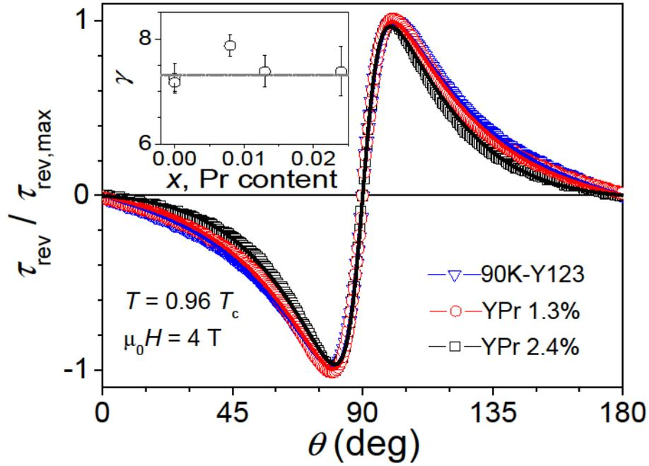
Fig. 3. Angular dependence of the normalized reversible torque and the corresponding fit of equation (1) to the data: 90K-Y123 (triangles), YPr 1.3% (circles), YPr 2.4% (squares). Inset: Dependence of the anisotropy on the Pr content for all crystals, the line corresponds to the averaged anisotropy parameters for crystals with  $\delta \approx 0.03$ .
