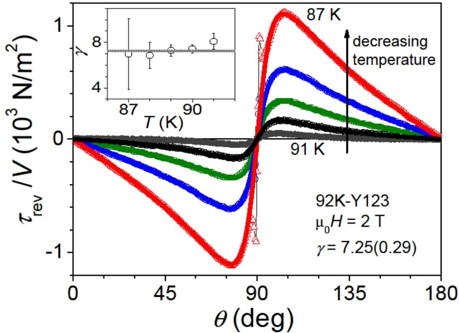
Fig. 4. Angular dependence of the reversible torque for 92K-Y123 at temperatures from 87 to 91 K at  $\mu_0 H = 2$  T and the corresponding fit of equation (1) to the data. Inset: Temperature dependence of the anisotropy parameter with maximal errors due to torque hysteresis. The line is a guide to the eye.
