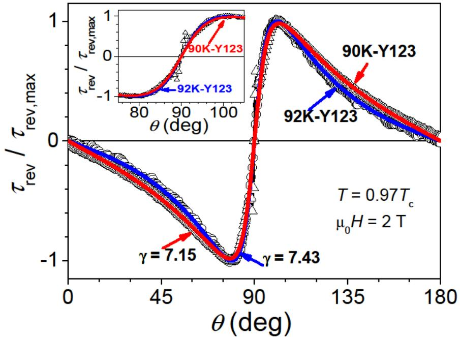
Fig. 2. Angular dependence of the normalized reversible torque for 90K-Y123 (triangles) and 92K-Y123 (circles) with fits of equation (1) to the data. Inset: the same dependence for angles close to 90 deg.
