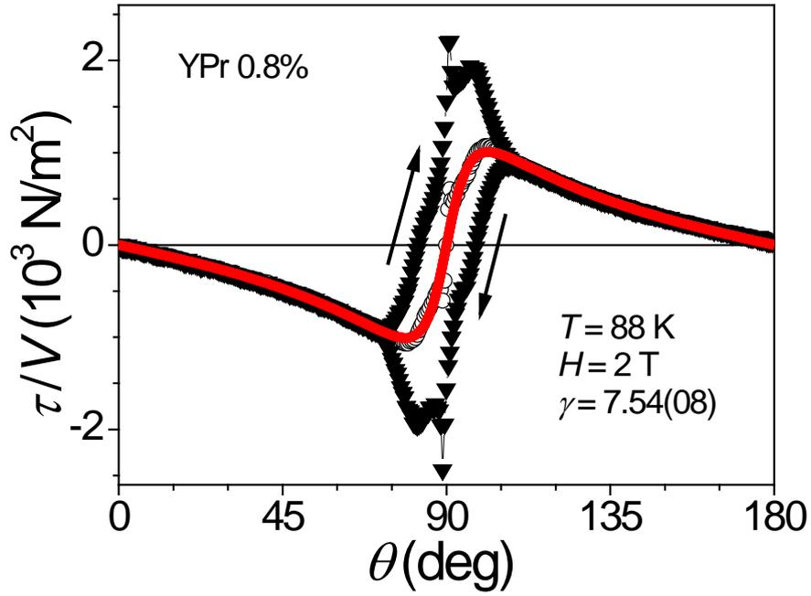
Fig. 1. Angular dependence of the torque for Y123 with 0.8% Pr content. Triangles denote the irreversible (clockwise and counterclockwise) and circles denote the reversible (averaged) torque. The solid line shows a fit of equation (1) to the data.
