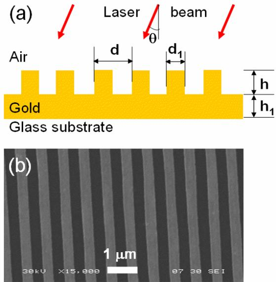
FIG. 1 (color online). Measured samples: (a). Schematic of the sample profile and the geometry of the laser beam incidence (red arrows). The two samples had the following dimensions. Sample 1:  $d = 705 \text{ nm}$ ,  $d_1 = 390 \text{ nm}$ ,  $h = 27 \text{ nm}$ ,  $h_1 = 35 \text{ nm}$ . Sample 2:  $d = 700 \text{ nm}$ ,  $d_1 = 365 \text{ nm}$ ,  $h = 50 \text{ nm}$ ,  $h_1 = 0$ . (b). SEM image of sample 2.
