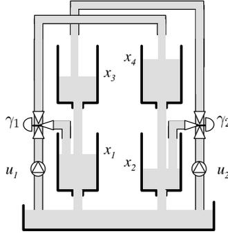
FIGURE 1. The quadruple-tank system.
