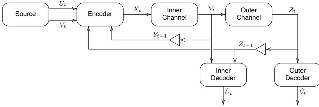
Fig. 1. A broadcast communication system with feedback
