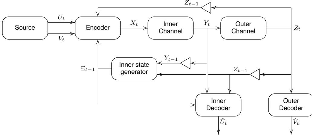
Fig. 3. The broadcast system with simplified encoder and inner decoder.
