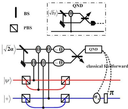
FIG. 1: (Color online) Schematic setup for entangler. Two qubus beams are coupled to the two single photons as indicated. The XPM phases  $\theta$  and two phase shifters  $-\theta$  are applied to the qubus beams. The QND module and the classical feedforward are used to make this operation to be deterministic. After that, an entangled state will be achieved.
