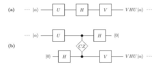
Figure 1: The Hadamard gadget for removal of intermediate H gates. (a)  $|\alpha\rangle$  represents a general input state to a gate U within the circuit that is followed by an intermediate H gate. (b) The lower line is a new ancillary qubit line. The original intermediate H gate may then be replaced by a new CZ gate, a post-selection (denoted by  $\langle 0|$ ) and two H gates that are now both at the ends of lines, as allowed in IQP circuit architecture.
