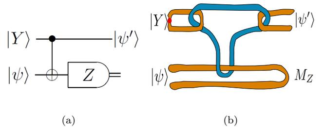
FIG. 3. (a) Gate teleportation circuit. A probabilistic phase gate K. Given the *magic state*  $|Y\rangle = \frac{1}{\sqrt{2}}(|0\rangle + i|1\rangle)$ , the gate teleportation circuit will return  $|\psi'\rangle = X^{M_Z} K |\psi\rangle$ , where  $M_Z \in \{0, 1\}$ . Similar results hold for  $\frac{\pi}{8}$  gates. (b) Topological gate teleportation circuit.
