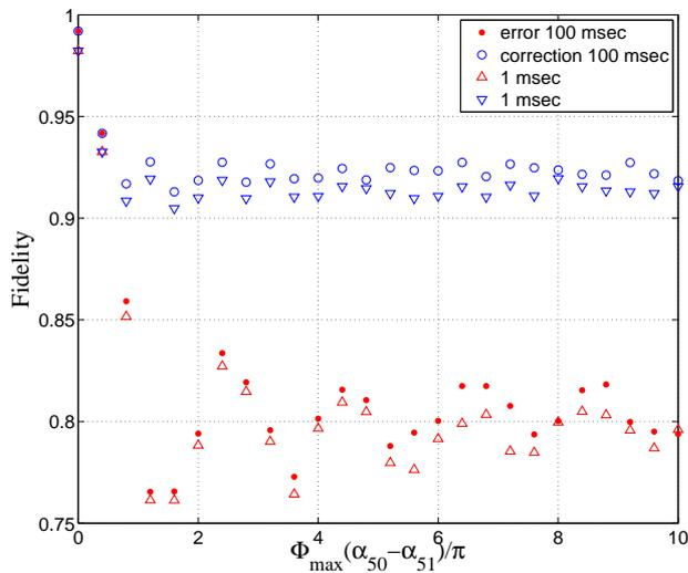
FIG. 4: (Color online) Comparison for two different cavity decay times  $T_{cav} = 100$  ms (blue circles for the QECC case and red dots with no QECC), and  $T_{cav} = 1$  ms (blue triangles for the QECC case and red triangles with no QECC). In both cases the initial state is with  $\alpha = \sqrt{60}$  and  $\beta = \sqrt{40}$ . The other parameters are the same as in Fig. 2
